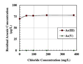
Figure 3. Effect of chloride on the adsorption of As(III) and As(V) by bauxite (temp.= $25^{\circ}$ C, initial As(V) 0.5 mg/L, pH=6, initial As(III) 0.5 mg/L, pH=7, adsorbent dosage =20g/L).
