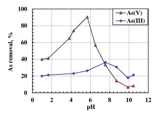
Figure 2. Effect of pH on the adsorption of As(III) and As(V) by bauxite with initial 0.5 mg/L As(V) or As(III).
