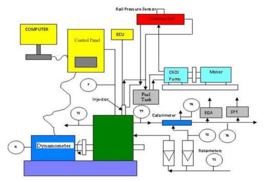
T1, T3 – Inlet Water Temperature, T2 – Outlet Engine Jacket Water Temperature T4 – Utlet Calorimeter Water Temperature, T5 – Exhaust Gas Temperature before Calorimeter T6 - Exhaust Gas Temperature after Calorimeter, F – Fluid Flow differential pressure Unit N – Speed Encoder, EGA – Exhaust Gas Analyser, SM – Smoke Meter
