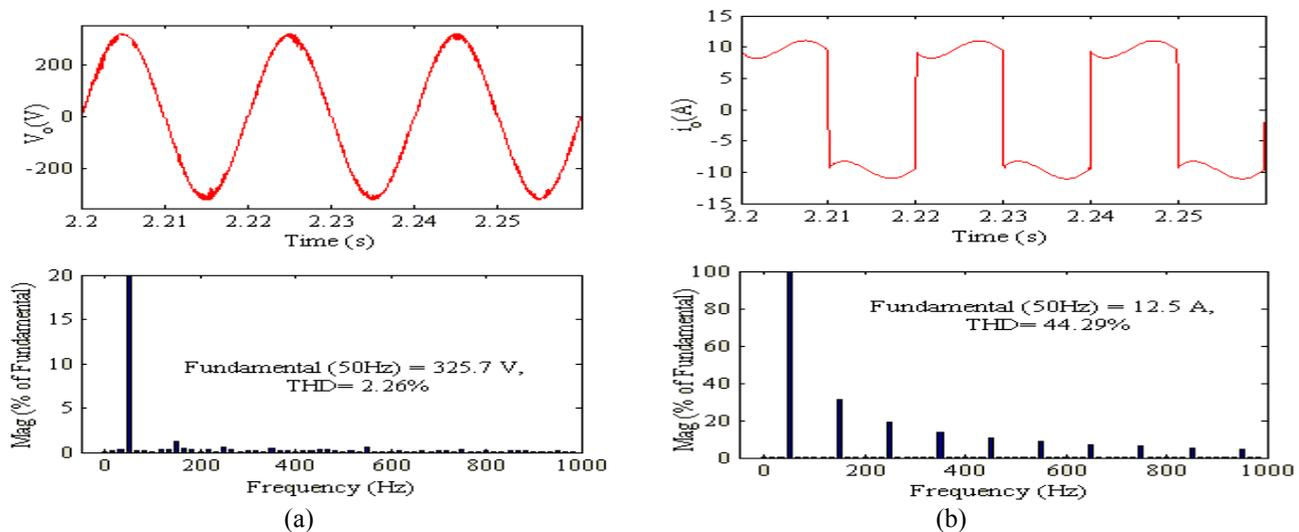
**Figure. 6** Harmonic spectra (a) load terminal voltage  $V_L$  (b) load current  $i_L$
