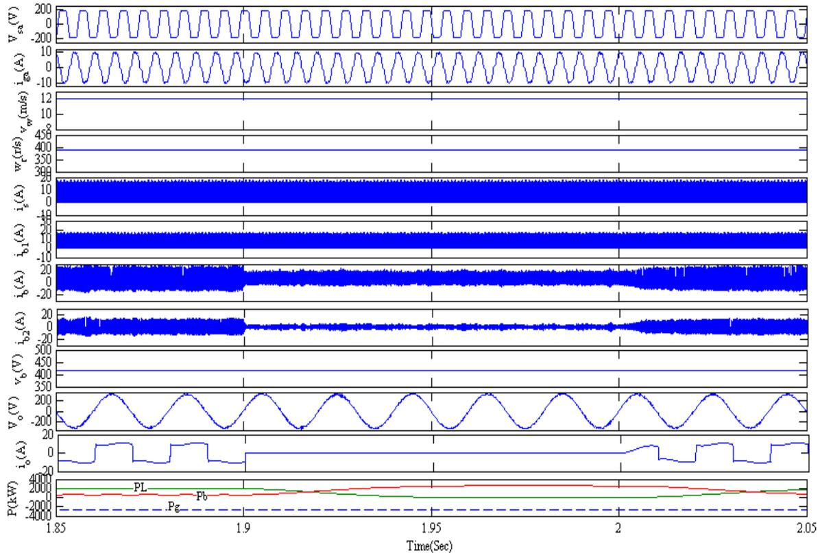
**Figure. 5** Performance of VFC at fixed wind speed (12 m/s) under non-linear load
