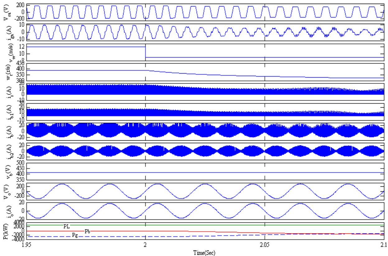
**Figure. 2** Performance of VFC under fall in wind speed (12 m/s-9 m/s) at fixed linear load
