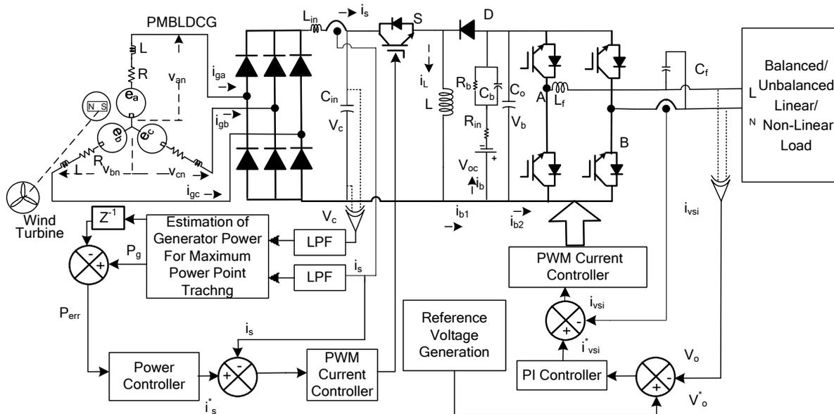
Figure. 1 Block diagram of system configuration of PMBLDCG based stand-alone WECS
