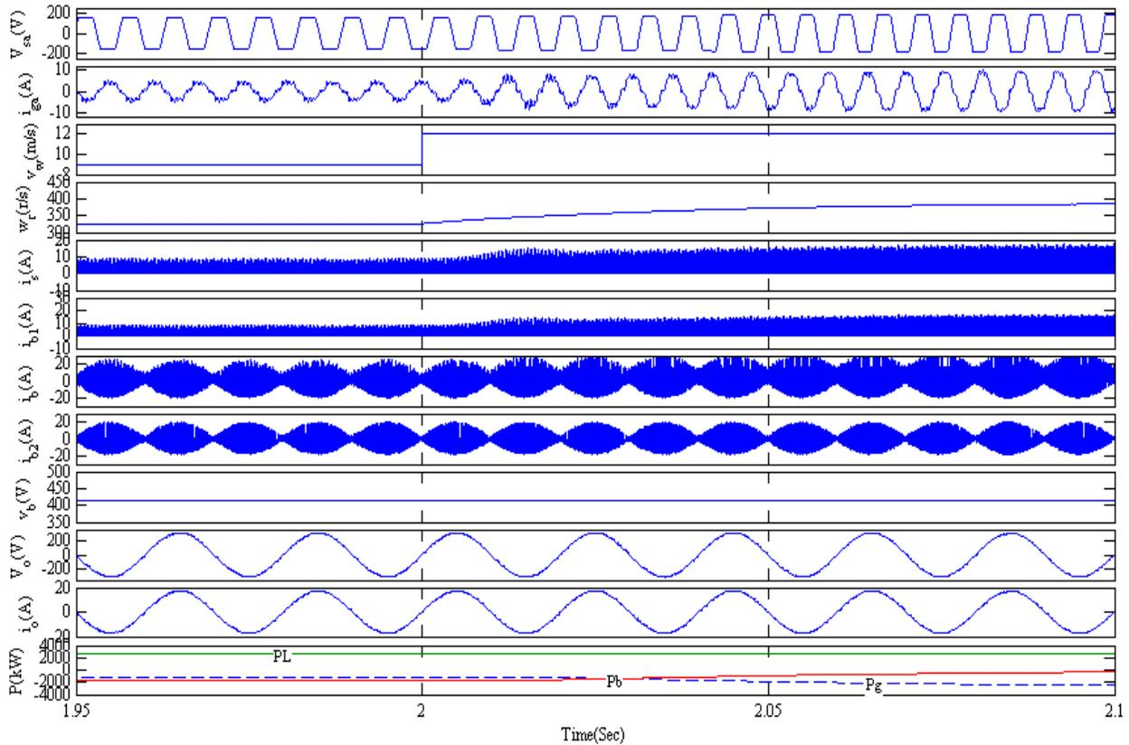
**Figure. 3** Performance of VFC under rise in wind speed (9 m/s-12 m/s) at fixed linear load
