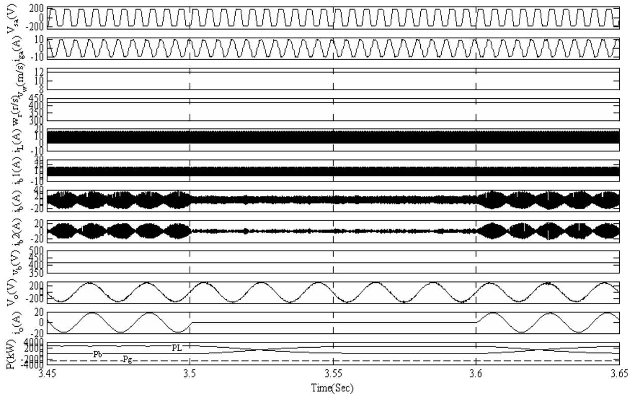
**Figure. 4** Performance of VFC at fixed wind speed (12 m/s) under linear load
