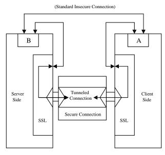
Figure 3. Tunneling Over Secure Connection
