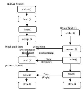
Figure 4.TCP/IP Client-Server Socket Programming Overview
