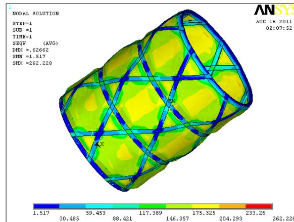
Figure 7. von Mises (equivalent) stress under ACPL
