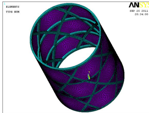
Figure 6. Mesh generation of stiffened cylinder with outer skin
