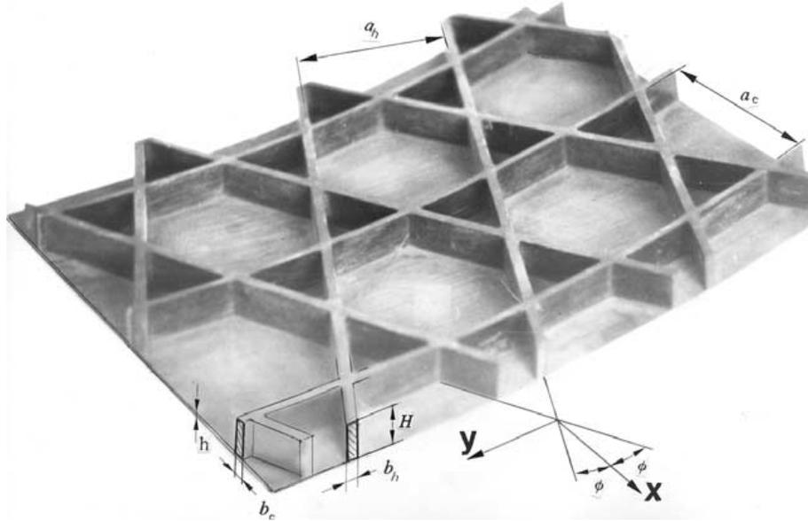
**Figure 1.** Parameters of a lattice structure (Vasiliev et al., 2001)
