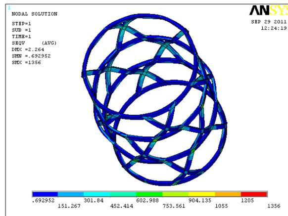
Figure 11. Equivalent (von Mises) stress distributions (first case study)
