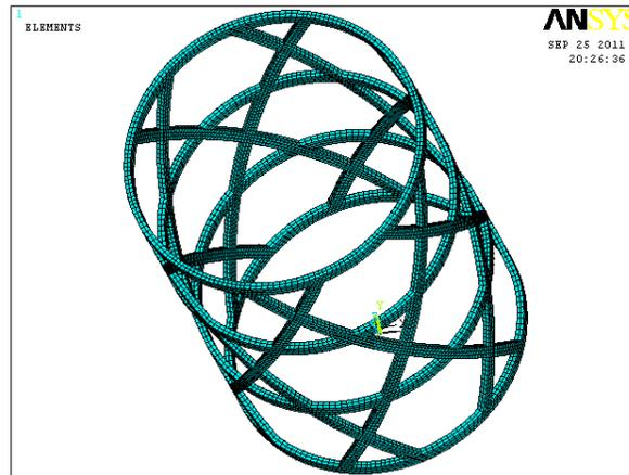
**Figure 4.** Mesh generation of stiffened cylinder without skins
