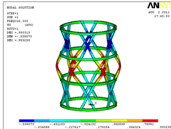
Figure 16. Buckling results ( $t = 0, H = 4\text{mm}$ ) for axial load
