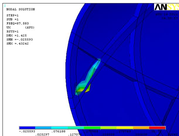
Figure 10. Stiffener crippling result example
