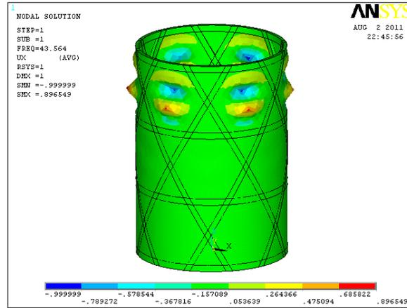
Figure 18. Buckling results ( $t = 0.8, H = 3.2\text{mm}$ ) for axial load
