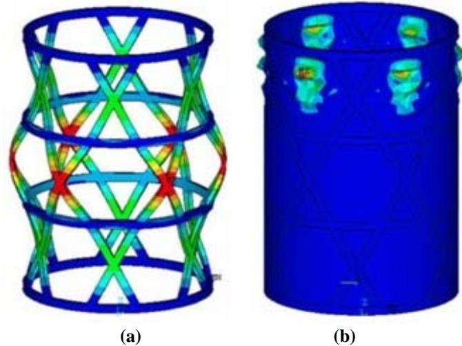
**Figure 19.** Typical buckled shapes by finite element modeling
