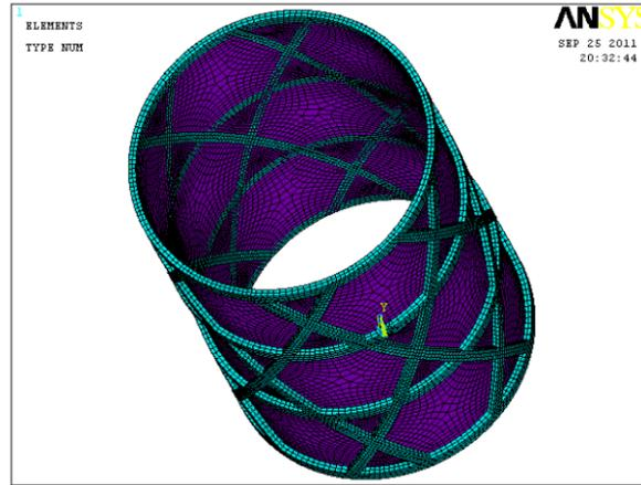
Figure 5. Mesh generation of stiffened cylinder with inner skin
