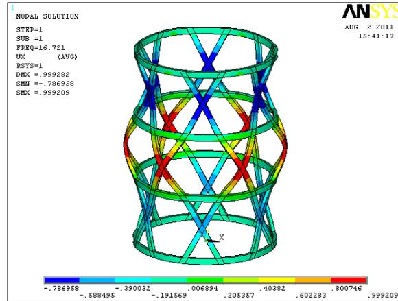
Figure 15. Buckling results ( $t = 0, H = 3.2\text{mm}$ ) for axial load
