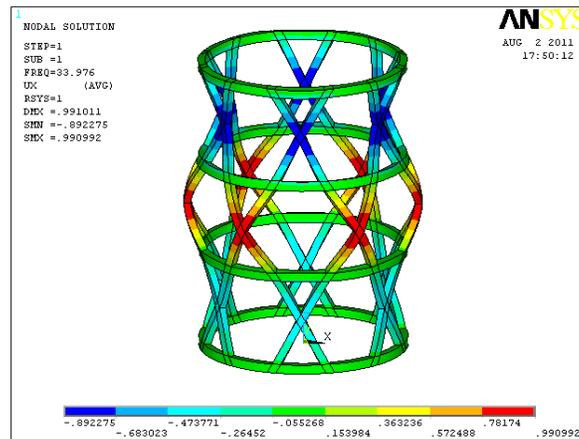
Figure 17. Buckling results ( $t = 0, H = 4.8\text{mm}$ ) for axial load
