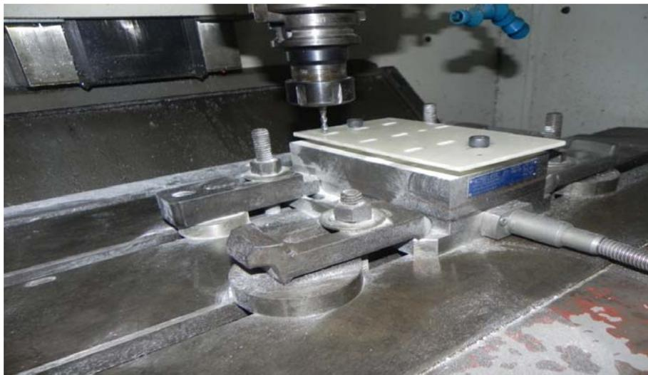
Fig. 3 Fixation of GFRP composite plate by using clamps in the machining centre.
