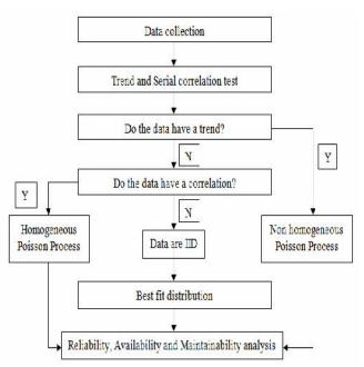
Figure 1. Step by step procedure of RAM analysis
