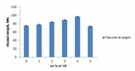
Figure 3. Flexural strength of CB-Epoxy composites for different weight percentage of CB
