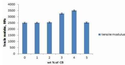
Figure 2. Tensile modulus of CB-Epoxy composites for different weight percentage of CB
