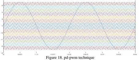
The technique uses a Sinusoidal wave of frequency 50 Hz as the reference signal that is compared with triangular carrier waves of frequency 2 kHz. The resultant PWM output then acts as gate driver signal for the MOSFETS.
