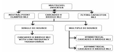
Figure 1. classification of multilevel inverters
