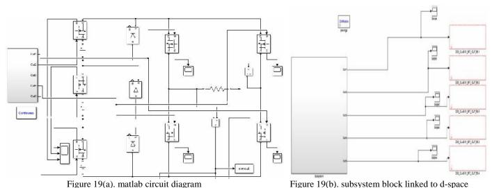
The PWM control signals are generated within a block subsystem and are fed to the gates of each MOSFET respectively. The signals generated using subsystem are shown in Figure 20 & 21.
