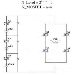
Figure 2. asymmetric h-bridge multilevel inverter
