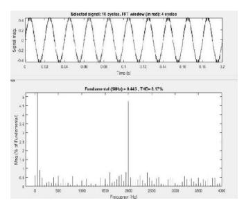
Figure 27. current thd for RL load (470 ohms, 20mh)
