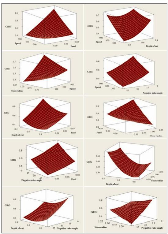
**Figure 7.** Response plots for GRG [Hold Values Speed 600; Feed 0.06; Depth of cut 0.6; Nose radius 0.8; Negative rake angle  $25^{\circ}$ ]
