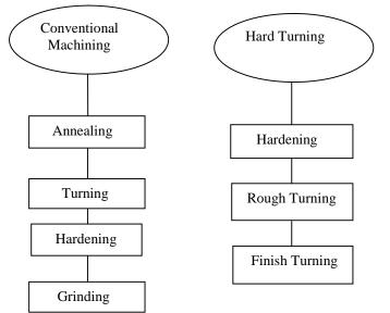
Figure 1. Distinction between conventional machining and hard turning (Dogra et al., 2010)
