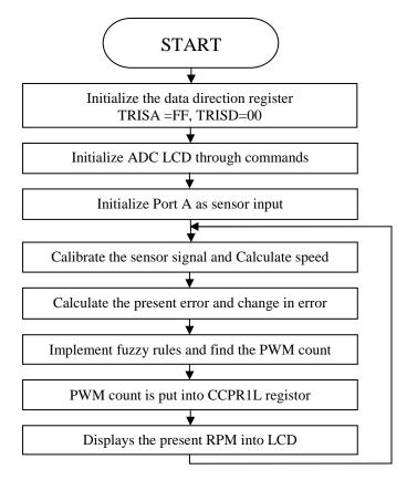
Figure 7. Program flow of DC motor control
