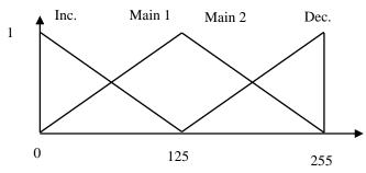
Figure 5. Fuzzification of binary count signal
