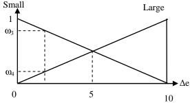
Figure 3. Fuzzification of 'error (e  $_{(n)}$ )' signar
