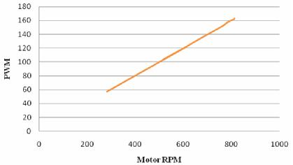
Figure 9. Graph between DC motor RPM and PWM
