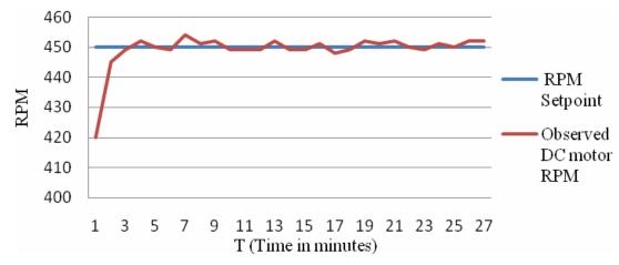
Figure 10. Graph between DC motor RPM and Time
