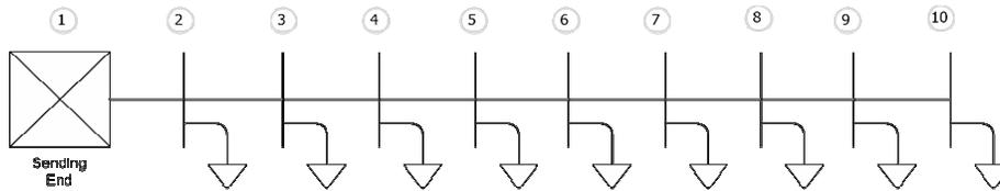
Figure3.One-line diagram of IEEE 10 bus RDS.
