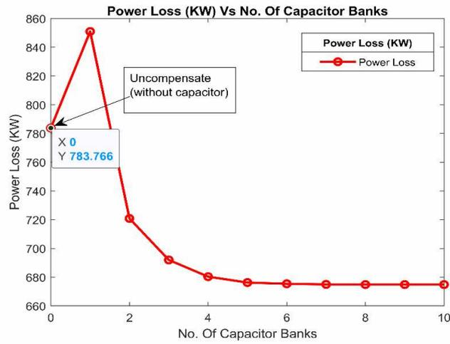
Figure 4. Power Loss (KW) Vs No. Of Capacitor Banks.
