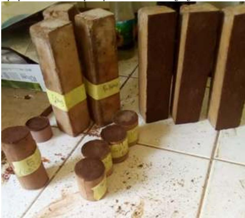
**Fig.1** Geopolymer mortar samples
