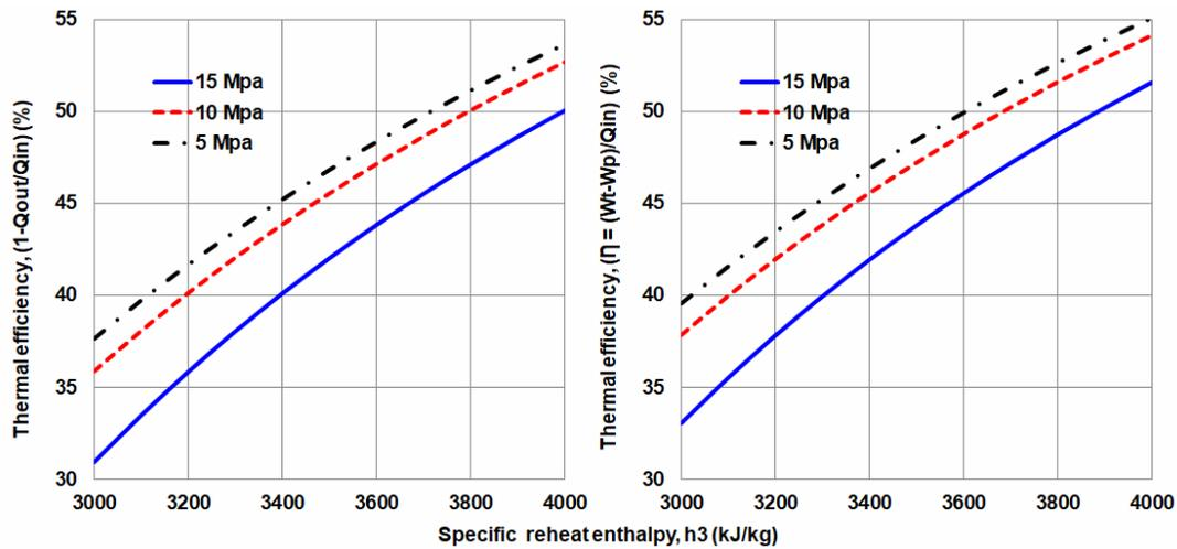
Figure 8. Effect of reheat intensity on the thermal efficiency of the steam power plant.
