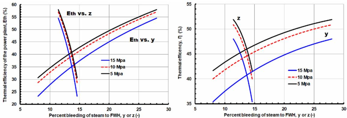
Figure 11. Variation of the steam power plant thermal efficiency ( $E_{th}$  and  $\eta_{th}$ ) with percent bleeding to the FWHs,  $y$  and  $z$ .
