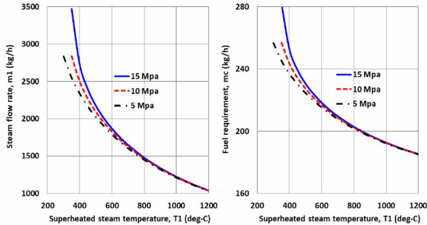
**Figure 5.** Effect of superheating temperature on the required steam flow rate into the high-pressure turbine and fuel requirements.
