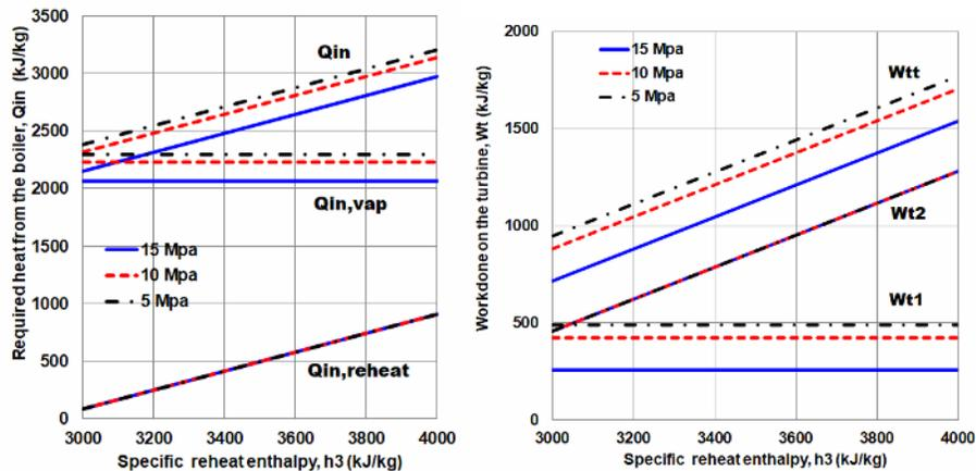
**Figure 6.** Effect of reheat intensity (heat input) on: (a) boiler heat requirement; (b) work done by steam on the turbine ( $W_{t1}$ ,  $W_{t2}$  and  $W_{tt}$ ).
