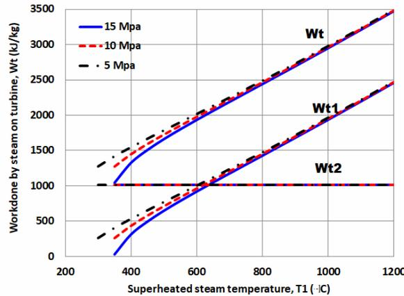
**Figure 4.** Effect of superheating temperature on the work done by steam on the turbine at different boiler pressures.
