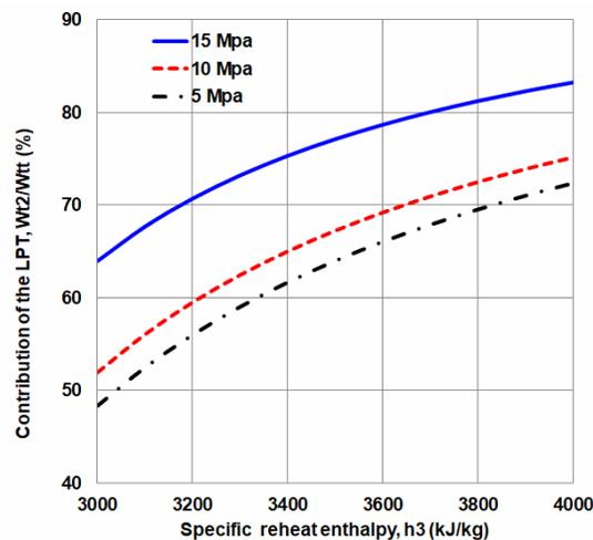
**Figure 7.** Variation of contribution of the low-pressure turbine on the total work done with increasing reheat intensity.
