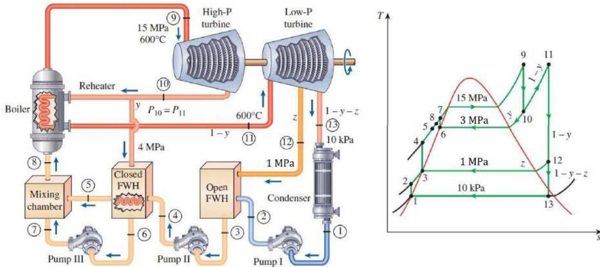
**Figure 2.** Schematic diagram of a double extraction regenerative reheat steam power plant with a T-s diagram.
