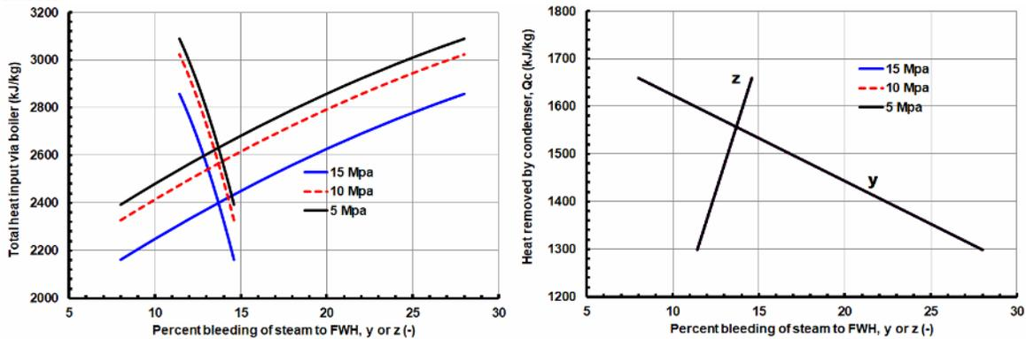
Figure 9. Effect of percent bleeding to the FWHs on: (a) the required heat input across the boiler,  $Q_{in}$ ; (b) condenser duty,  $Q_c$ .
