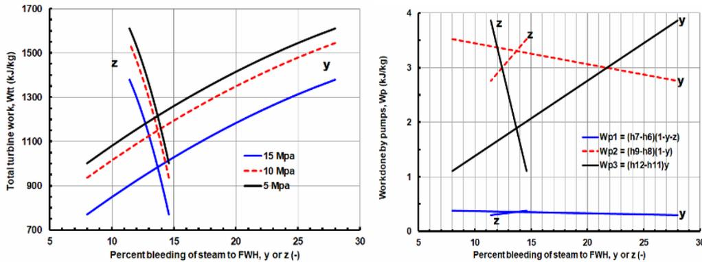
Figure 10. Effect of percent bleeding to the FWHs on: a) the total work done on the turbine; b) the work done by condensate pumps.
