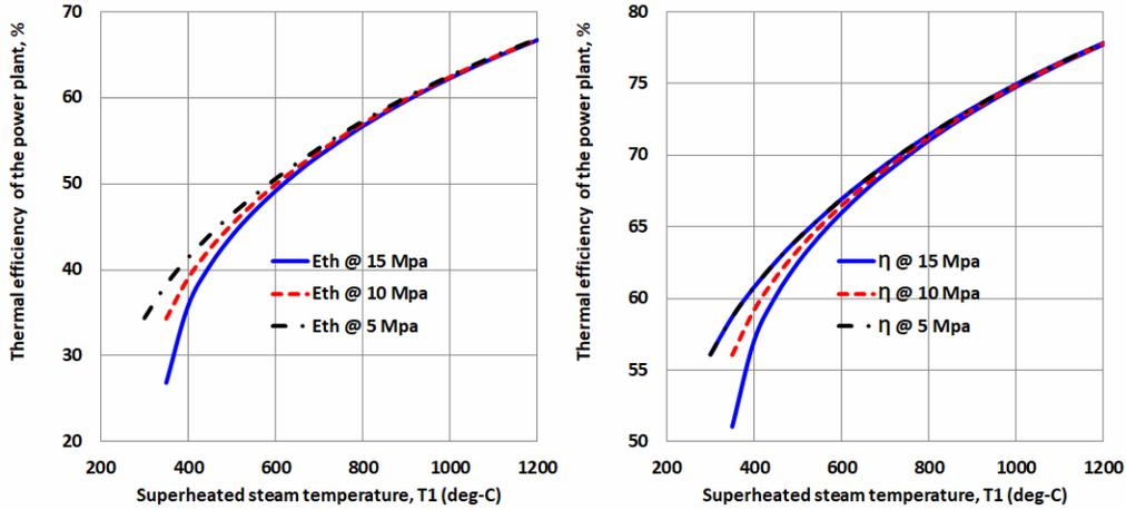
**Figure 3.** Effect of superheating temperature on the thermal efficiency of the steam power plant.
