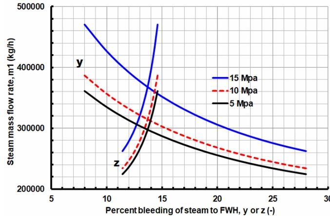
**Figure 12.** Variation of the required steam mass flow rate into HPT with percent bleeding to the FWHs.
