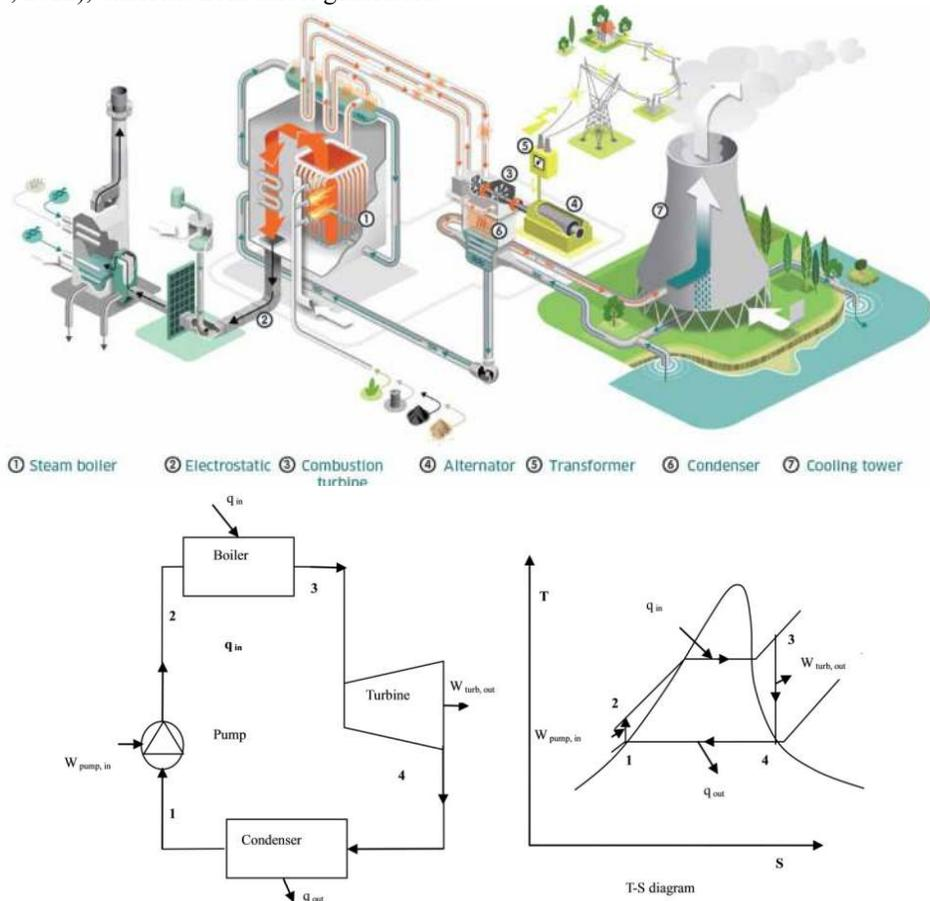
**Figure 1:** Schematic of Rankine cycle steam power plant with the corresponding simplified ideal process flow and T-s diagrams (Vundela *et al.*, 2010).
