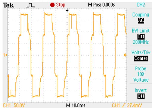
Figure 10. Non-adjacent line voltage for 144° conduction mode with dc link voltage equal to 180 V.
