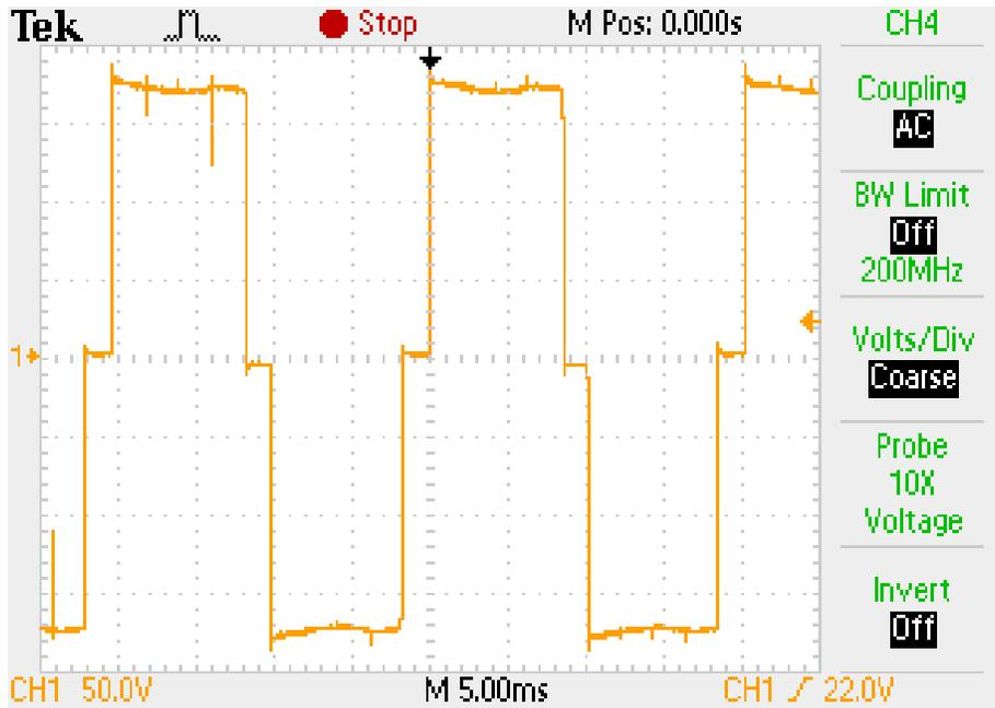
Figure 6. Non-adjacent line voltage for 180° conduction mode with dc link voltage equal to 180 V.
