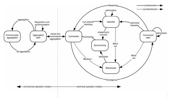
Figure 3. Control modes and transition for subgrid operation
