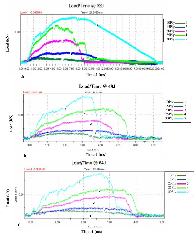
Figure 1. Curves of impact load versus time of woven natural silk fabric composite plates. (a) Impact load of 32J (b) Impact load of 48J (c) Impact load of 64J
