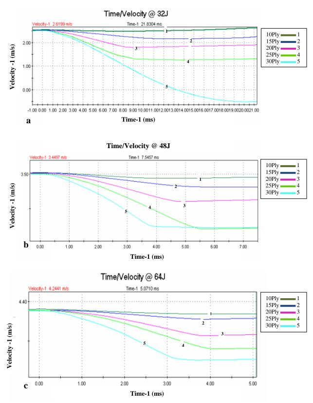
Figure 6. Velocity - time curve for different ply at impact energy level (a) 32J (b) 48J (c) 64J
