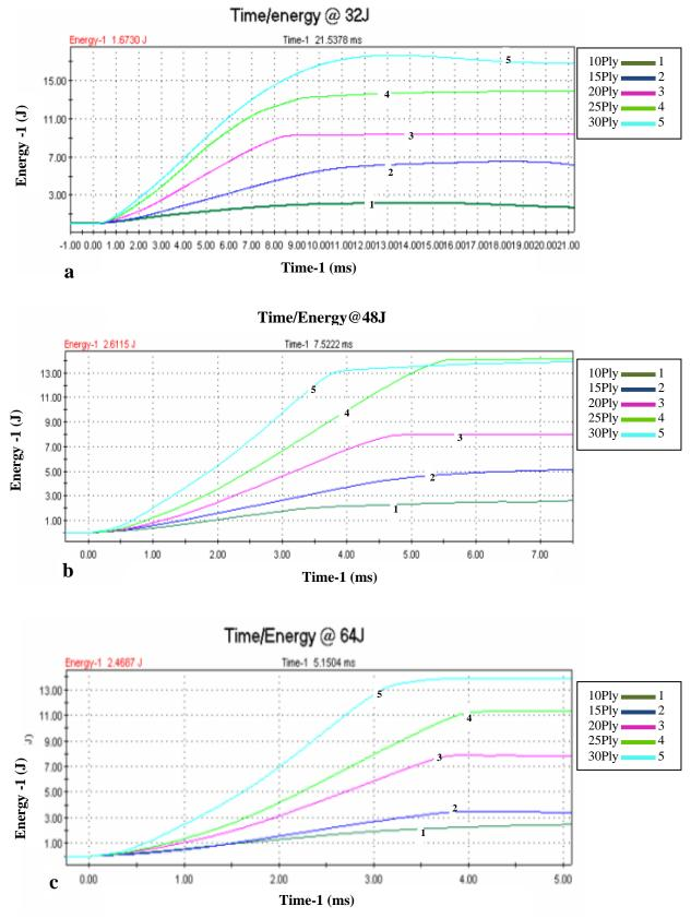
Figure 4. Energy absorption versus time curves under: (a) 32J (b) 48J and (C) 64J
