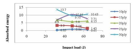
Figure 5. The absorption capability comparison of each composite category with increasing load
