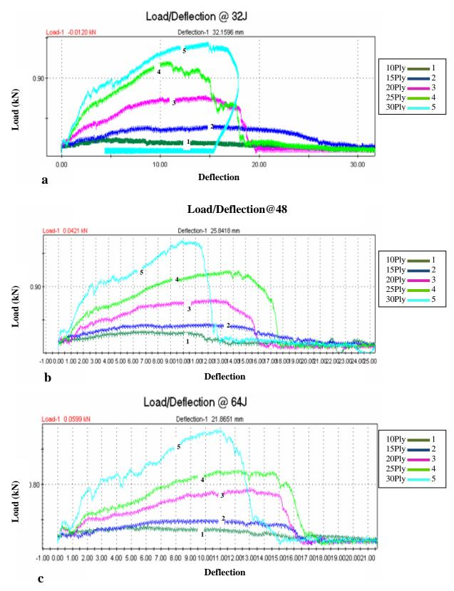
Figure 3 Load – deflection curves under (a) 32J (b) 48J (c) 64J impact energy.
