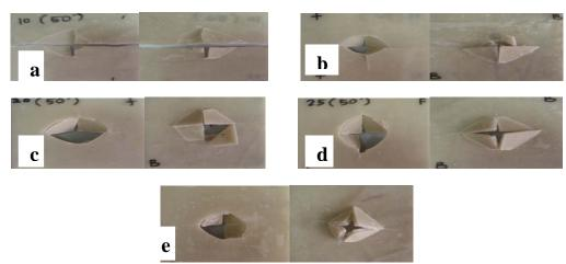
Figure 10. Specimens under 64J impact loading. (a) 10ply (b) 15ply (c) 20ply (d) 25ply (e) 30ply
