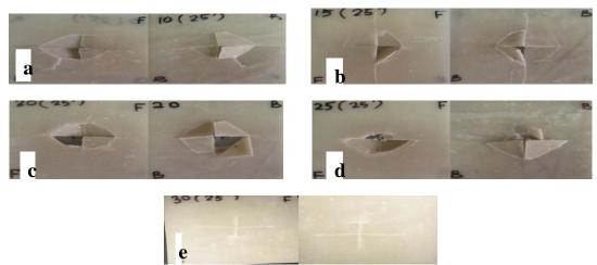
Figure 8. Specimens under 32J impact loading. (a) 10ply (b) 15ply (c) 20ply (d) 25ply (e) 30ply
