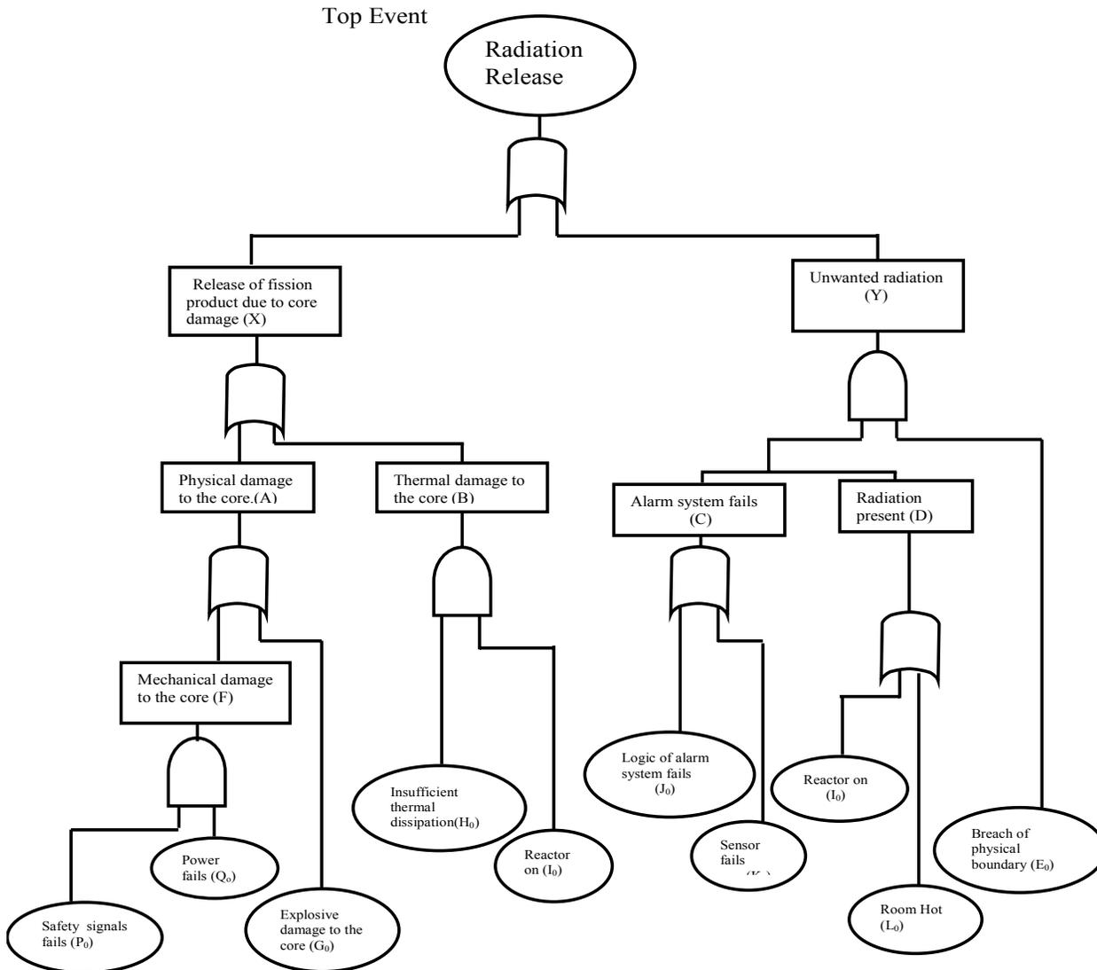
**Figure 1. Fault tree of Nuclear Power Plant**
