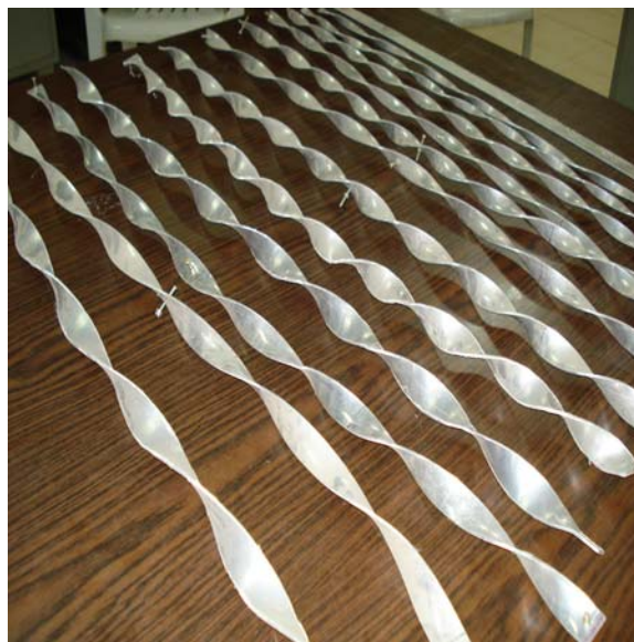
Figure 2: Photographs of twisted tape inserts
