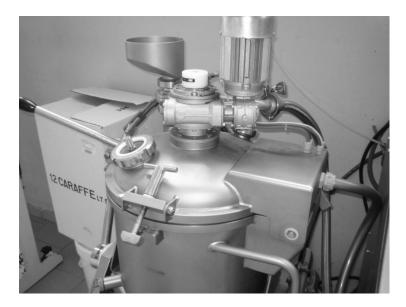
Figure- 3 Refrigerated vacuum milling chamber
