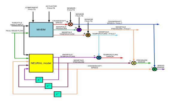
Figure 7. The information flow for the fault detection.
