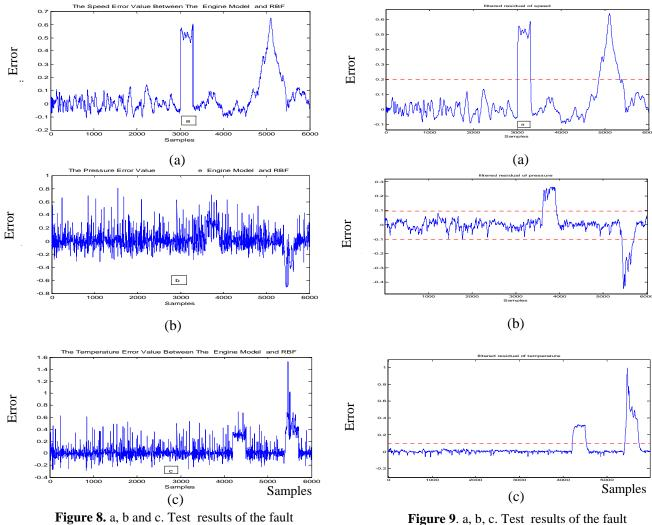
detection of speed, pres. & tem. respectively before filtering.
