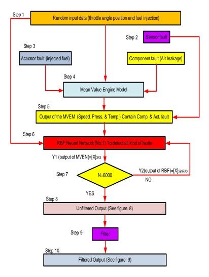
Figure 6. Flow chart of fault detection.
