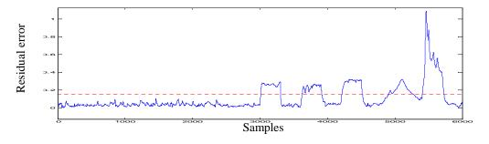
Figure 10. The residual error of the fault detection after filtering with 12 hidden nodes.
