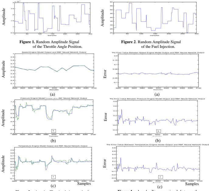
Figure 3, a, b and c. The simulation result of the speed, pressure and temperature engine model output and the RBF neural networks output respectively.
