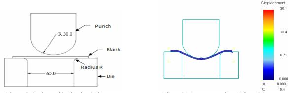
Figure 1: Tools used in the simulations
