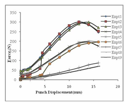
Figure 4: Deformed cup height vs Punch force
