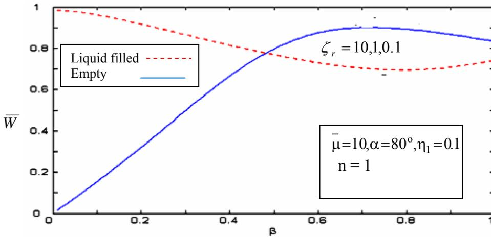
Figure 6 Radial displacement ( $\bar{W}$ ) vs. wave number ( $\beta$ ) with  $\Gamma_r = 0.1,1,10$  as parameter
