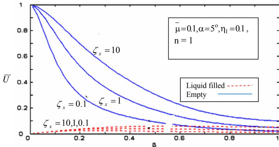
Figure 8. Axial displacement ( $\bar{U}$ ) vs. wave number ( $\beta$ ) with stiffness coefficient  $\zeta_x = 0.1, 1, 10$  as parameter
