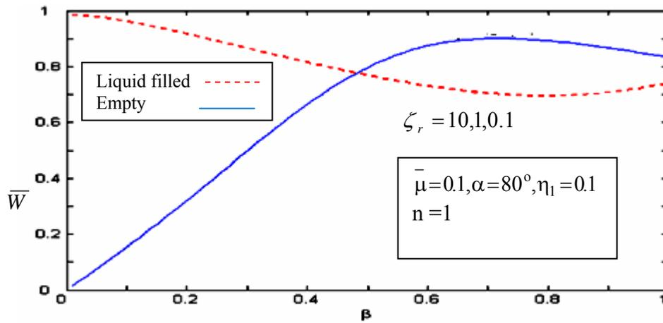
Figure 4. Radial displacement ( $\bar{W}$ ) vs. wave number ( $\beta$ ) with damping coefficient  $\Gamma_r = 0.1, 1, 10$  as parameter
