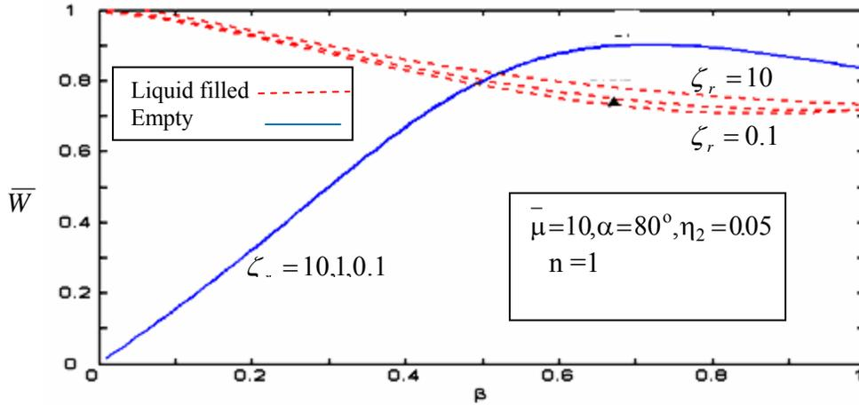
Figure 5. Radial displacement ( $\bar{W}$ ) vs. wave number ( $\beta$ ) with damping coefficient  $\Gamma_r = 0.1,1,10$  as parameter
