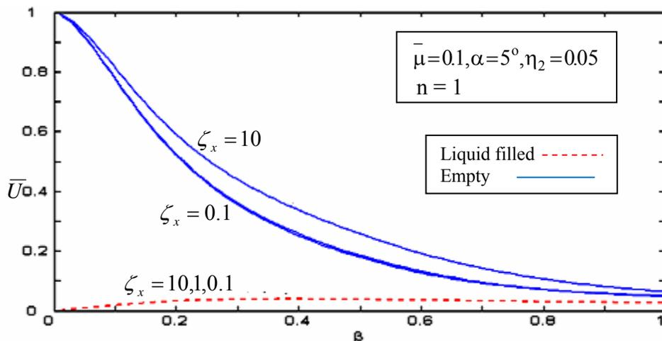
Figure 7. Axial displacement ( $\bar{U}$ ) vs. wave number ( $\beta$ ) with stiffness coefficient  $\zeta_x = 0.1, 1, 10$  as parameter
