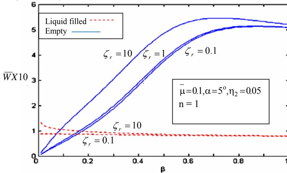
Figure1. Radial displacement ( $\bar{W}$ ) vs. wave number ( $\beta$ ) with stiffness coefficient ( $\zeta_r$ ) as parameter
