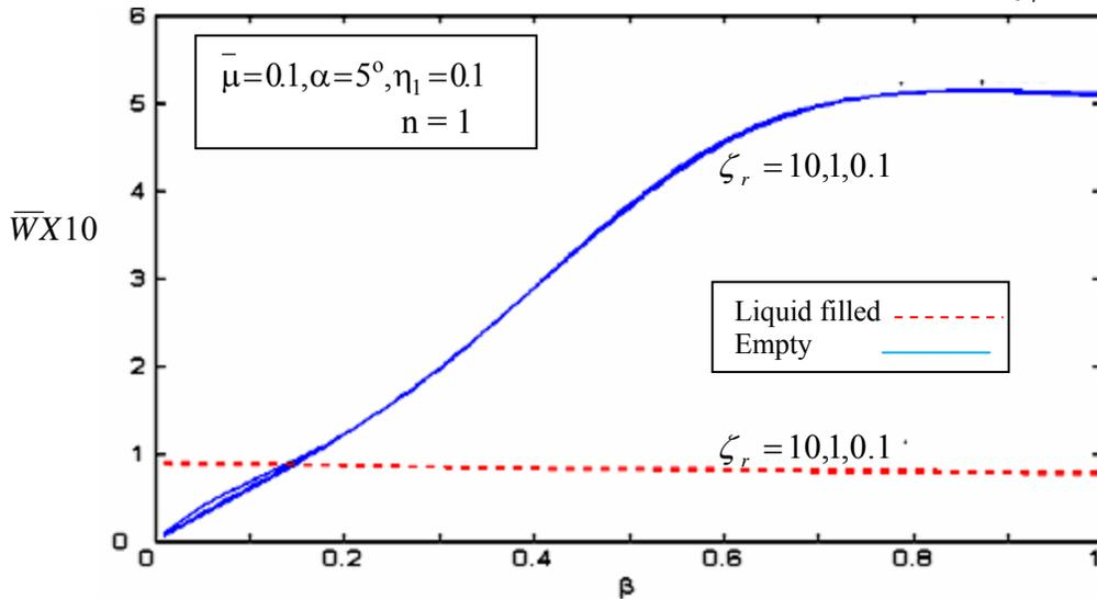
Figure 2. Radial displacement ( $\bar{W}$ ) vs. wave number ( $\beta$ ) with stiffness coefficient  $\zeta_r = 0.1, 1, 10$  as parameter
