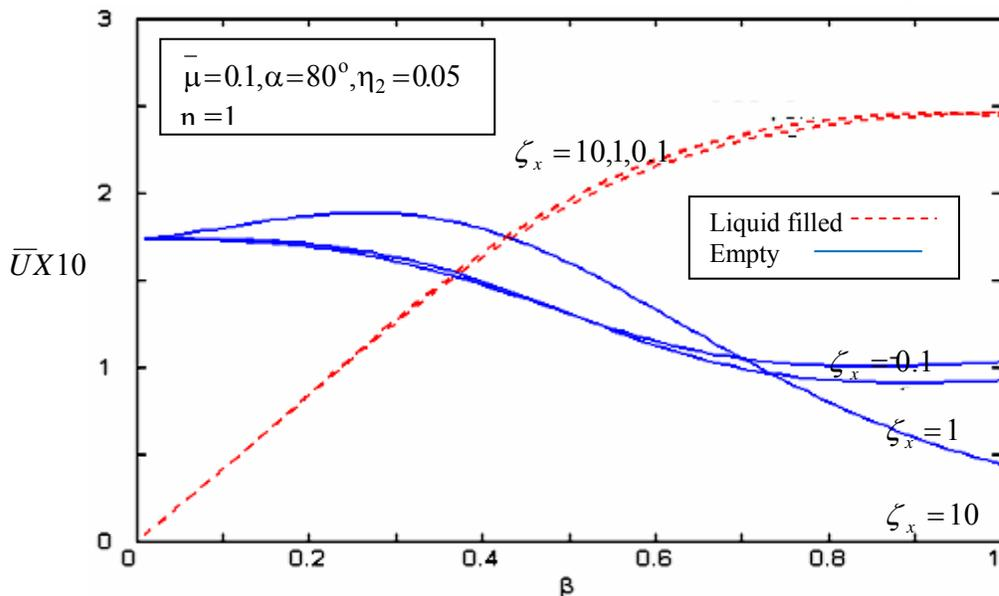
Figure 9. Axial displacement ( $\bar{U}$ ) vs. wave number ( $\beta$ ) with stiffness coefficient  $\zeta_x = 0.1, 1, 10$  as parameter
