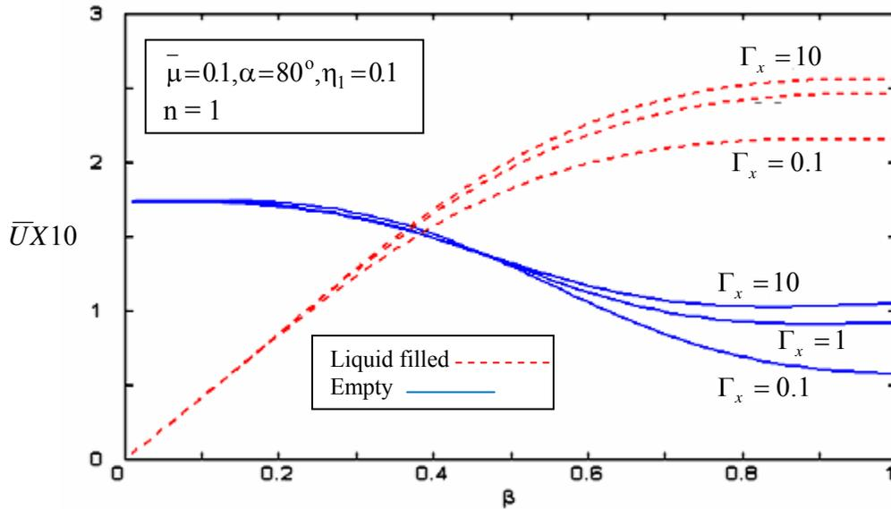
Figure 10. Axial displacement ( $\bar{U}$ ) vs. wave number ( $\bar{\beta}$ ) with damping coefficient  $\Gamma_x = 0.1, 1, 10$  as parameter
