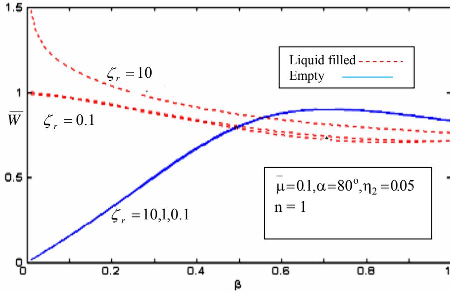
Figure 3. Radial displacement ( $\bar{W}$ ) vs. wave number ( $\beta$ ) with stiffness  $\zeta_r = 0.1, 1, 10$  as parameter
