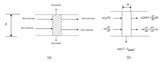
Heat energy converted in the left face + heat energy conducted in the left face = heat energy converted out of the right face + heat transfer by convection out of the top and bottom faces of the liquid and conduction between the mould and the liquid surfaces.
