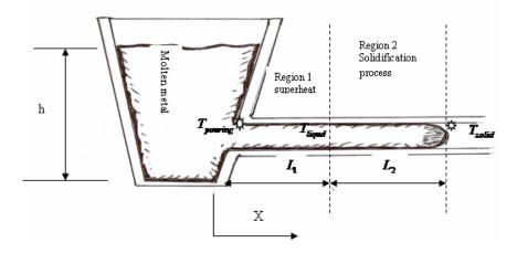
Figure 1: Mathematical geometry used to develop the analytical model
