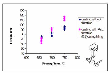
Figure 15: The fluidity of A356 alloy as a function of pouring temperature in the flowability filling type, according to the vibration techniques used during filling and gravity pouring
