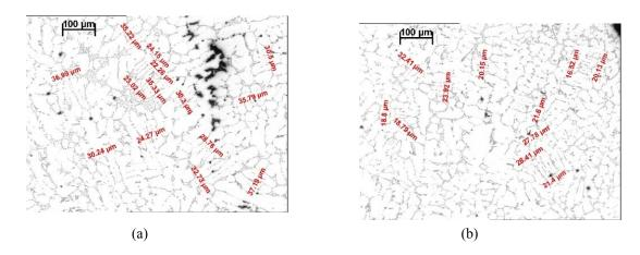
Figure 14 Typical mid-thickness strip microstructures observed at the flow tips of (a) castings filled without vibration and (b) castings filled with 0.8g acceleration (pouring temperature, thickness 0.75mm,750°C; mould temperature 420°C; metal head 170mm).
