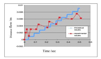
Figure 8 : Comparison between the experimental results and theoretical results of flow velocity of mercury in a strip of thickness 0.060mm, frequency 20 Hz, amplitude 0.5mm
