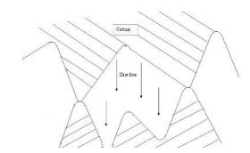
Figure 10: Metal-mould interfaces at the second stage (air gap forming).
