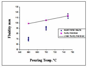
Figure 16 shows the relationship between the fluidity and the pouring temperature, casting without vibration, in a  $0.75^{\pm 0.05}$  mm channel. A theoretical line is obtained from the heat loss model.
