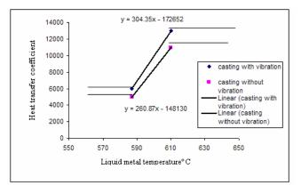
Figure 13: The variance of the calculated heat transfer coefficient with the temperature of the liquid metal
