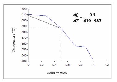
Figure 4: Temperature versus fraction solid in the AlSi7% alloy
