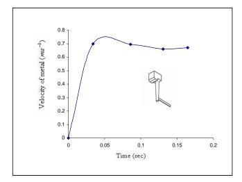
Figure 5: Velocity measurements, flowability filling condition, piece thicknesses 0.75mm, mould Temperature 450°C, pouring Temperature 750°C, and metal head 170mm
