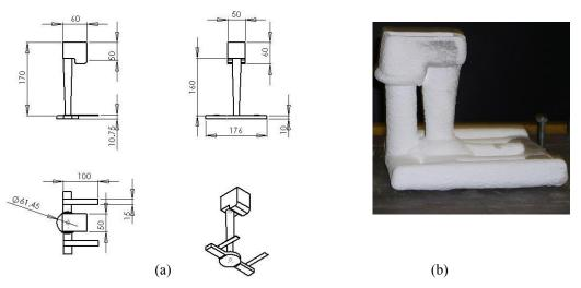
Figure 7 (a) Mould design for fluidity test strip thickness 0.75mm metal height 170 mm, pouring temperature 450°C, mould temperature 660°C-700C (b) ceramic mould
