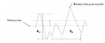
Figure 12 Schematic to show the definition of the surface roughness parameter.
