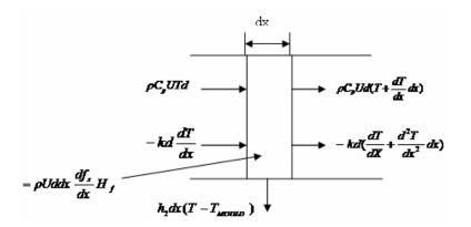
Figure 3: Elemental volume defined for energy analysis in the latent heat region (Al-Sammara and Dows, 1996).
