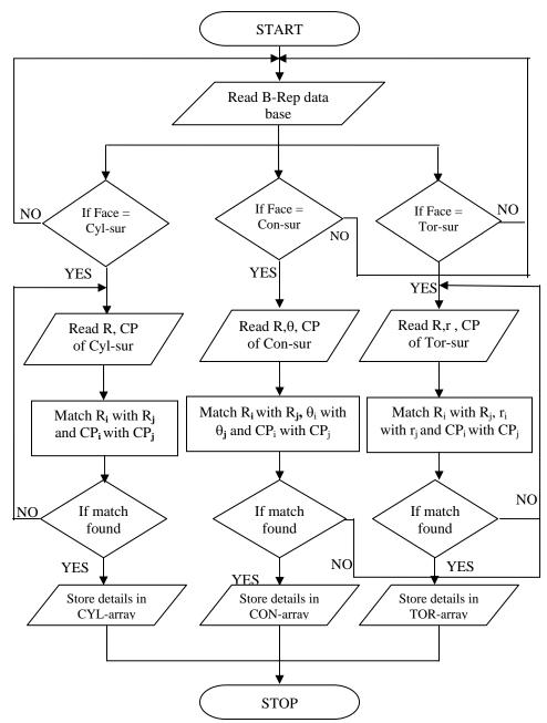
Figure 5. Algorithm for recognizing primary turning features
