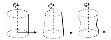
(a) Cylinder (b) Cone (c) Surface of Revolution
