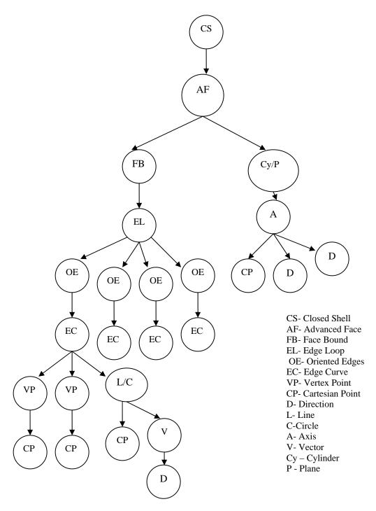
Figure 3. Structure of STEP file
