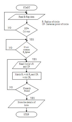
Figure 6. Radial hole recognition algorithm
