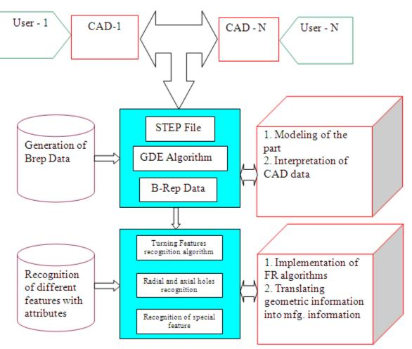
Figure 2. Methodology to recognize different turning features
