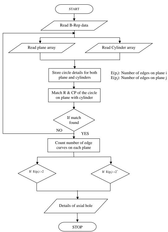
Figure 7. Algorithm for recognizing axial holes in rotational parts
