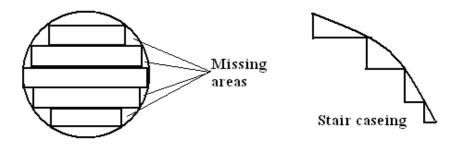
Figure 10: Stair case effect due to higher slice thickness
