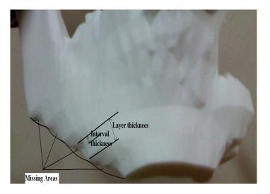
Figure 5: RP model of 5mm layer thickness and 1mm interval thickness
