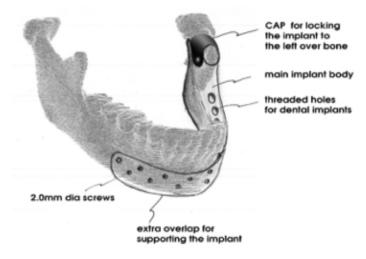
Figure 3: Arrangement of titanium plate on mandible of RP model
