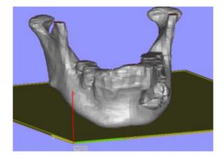
Figure 11: Orientation of part on RP machine
