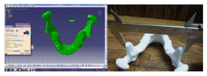
Figure 12: CAD model and Rapid Proto model Measurements are measured on CATIA & Callipers
