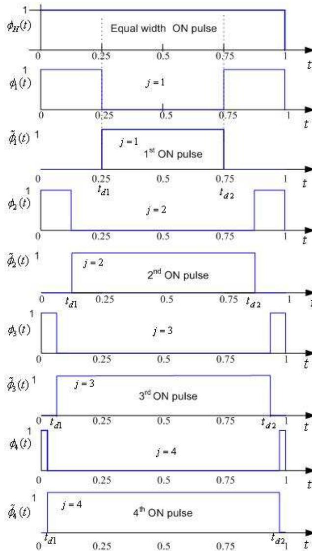
**Figure 2.** Variable width switching pulse generation using analysis function & synthesis scaling function at normalized time scale
