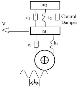
Figure 1: TDOF model of car and car seat
