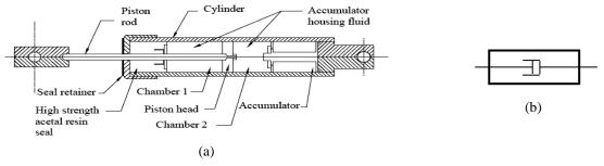
Figure 3: (a) Construction and (b) Mathematical Model of viscous damper (Symans and Constantinou, 1998)
