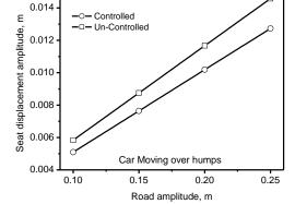
**Figure 7:** Variation of peak seat displacement with car velocity when employing LVD
