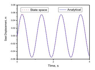
Figure 2: Displacement of the car moving over a sinusoidal road profile
