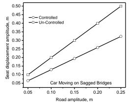
**Figure 10:** Variation of peak seat displacement with road amplitude when employing SAVFD
