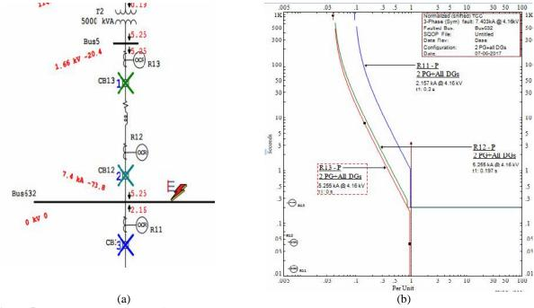
**Figure 5**. Fault at Bus 632 for Config. 2 (PG +All DGs): (a) Operating sequence One Line Diagram (OLD), (b) Time Current Characteristics (TCC)
