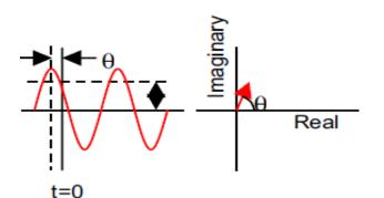
Figure 1: Definition of a Phasor, a complex number representation of a constant pure sinusoid.
