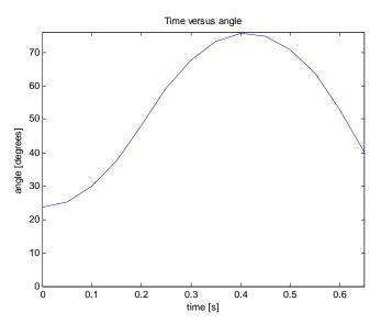
Figure 19: rotor angle against time for a stable case.
