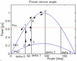
Figure 6: Power transfer before, during and after a fault close to the turbine-generator.
