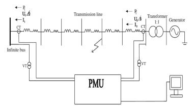
Figure 8: Simulated power system model (Berkestedt, 2007).
