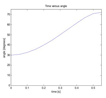
Figure 14: rotor angle against time for an unstable case.
