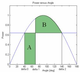
Figure 7: Equal-area criterion with an acceleration area A and a decelerating area B (Berkestedt, 2007).
