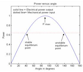
**Figure 5:** Input (dashed) and Output (solid) power of turbine generator.
