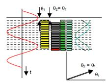
Figure 3: Recursive estimation of phasors from sampled data with moving window DFT.
