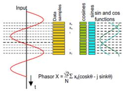
Figure 2: Estimation of phasors from sampled data using Discrete Fourier Transform.
