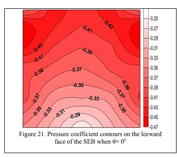
The CFD results presented thus far are not as good as might be hoped, although they do display the correct magnitude and trends in many cases. It was apparent that none of the models tested could accurately predict the experimentally obtained leeward pressure distribution.
