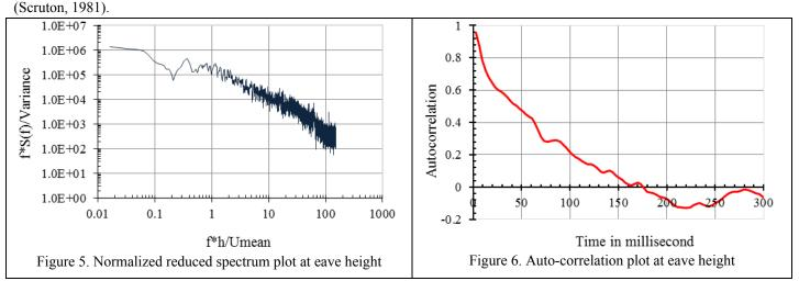
where, U is the mean wind speed,  $\tau$  is the time and  $\int_{0}^{\infty} R(\tau) d\tau$  is the area under the auto-correlation curve as shown in Figure 6
