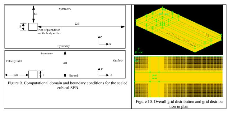
Wall boundary conditions were specified using wall functions on the surface of the building model. Viscous boundary layers were generated on the surface of the SEB with 20 grid layers. The height of the first cell of the boundary layer were chosen to be 0.084*mm* to ensure wall unit  $y^+ \approx 1 \left( y^+ = \frac{\rho u y}{\mu} \right)$  for LES and a wall unit  $y^+ < 5$  were used for all the RANS turbulence models.
