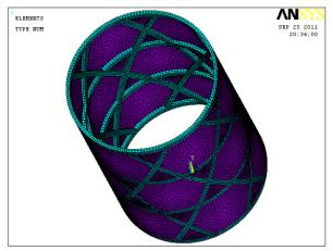
Figure 6. Mesh generation of stiffened cylinder with outer skin
