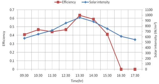
Figure 8. Variation of efficiency along with variation of solar intensity for solar air collector without reflector at 45° tilt angle
