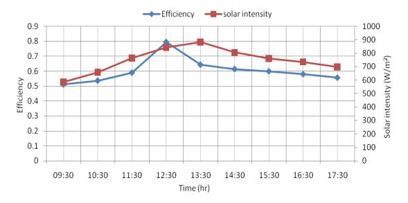
Figure 14. Variation of efficiency along with variation of solar intensity for solar air collector with reflector at 30° tilt angle
