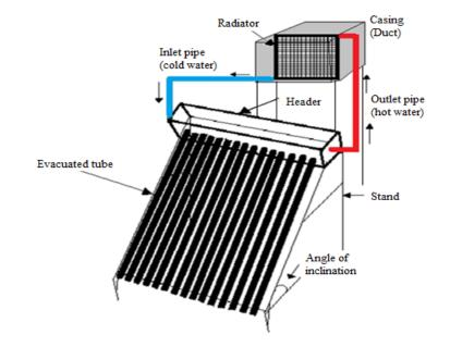
Figure 1. Schematic diagram of the evacuated tube solar air collector.
