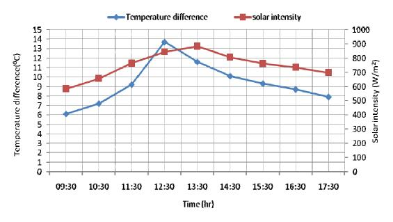
Figure 13. Variation of temperature difference of air along with variation of solar intensity for solar air collector with reflector at 30° tilt angle
