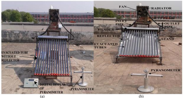
Figure 2. Photograph of experimental setup at tilt angle (a) without reflector, (b) with reflector
