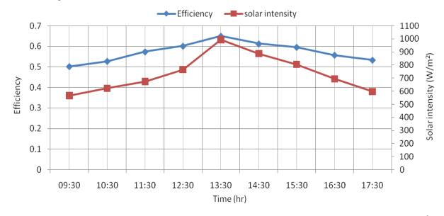
Figure 12. Variation of efficiency along with variation of solar intensity for solar air collector without reflector at 30° tilt angle
