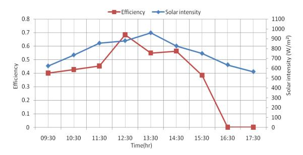
Figure 10. Variation of efficiency along with variation of solar intensity for solar air collector with reflector at 45° tilt angle
