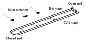
Figure 6. Thermosyphon phenomenon inside the evacuated tube
