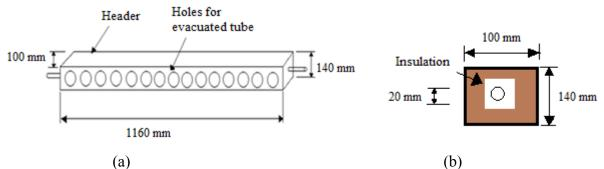
Figure 4. Schematic diagram of (a) complete header, (b) cross-sectional view of header
