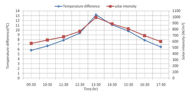
hr, solar intensity was also maximum at this time. In this case, the maximum temperature difference of the air is more than the case of solar air heater without reflector at 45° tilt angle of solar collector.
