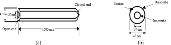
Figure 3. (a) Schematic diagram of one ended evacuated tube along the length (b) Schematic diagram of cross-section of one ended evacuated tube
