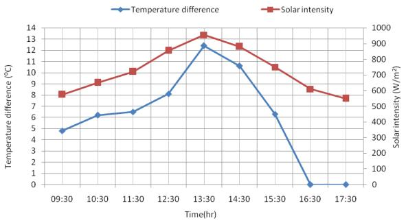
Figure 7. Variation of temperature difference of air along with variation of solar intensity for solar air collector without reflector at 45 tilt angle
