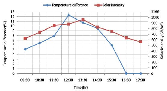
Figure 9. Variation of temperature difference of air along with variation of solar intensity for solar air collector with reflector at  $45^{\circ}$  tilt angle
