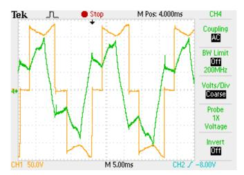
Figure 19. Non-adjacent line voltage Vac and  $I_b$  (180° conduction mode).
