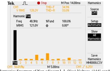
Figure 23. Harmonics Spectrum of Non-adjacent L-L (Vac) Voltage (144° conduction mode)
