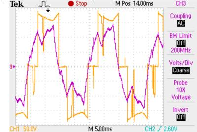
Figure 22. Non-adjacent L-L (Vac) Voltage and Line Current (I<sub>b</sub>) (144° conduction mode)
