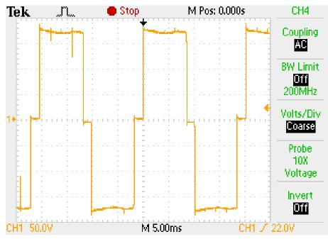
Figure 6. Non-adjacent line voltage for 180° conduction mode with dc link voltage equal to 180 V.
