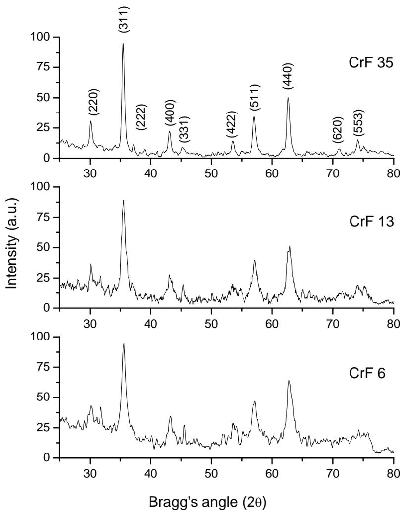
**Figure 1:** XRD pattern of 6 nm, 13 nm and 35 nm size CrF nanoparticles
