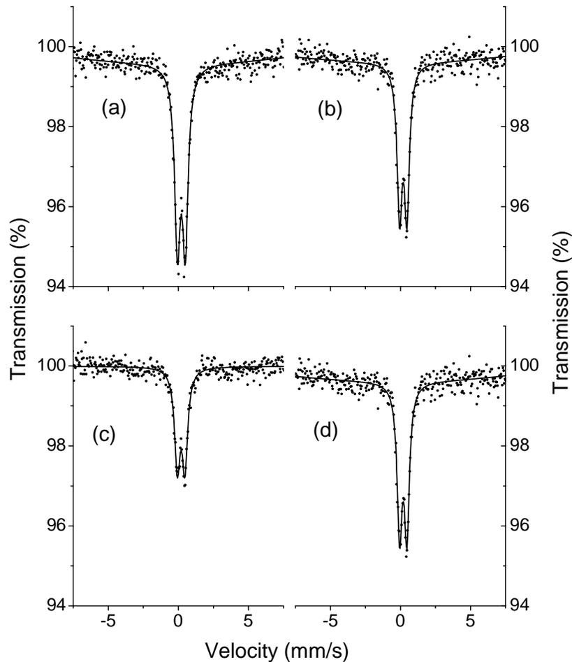
**Figure 7:** Mössbauer spectra of nanosize CrF samples (a) 6 nm, (b) 13 nm and (c) 35 nm at room temperature and (d) 13 nm at 16 K
