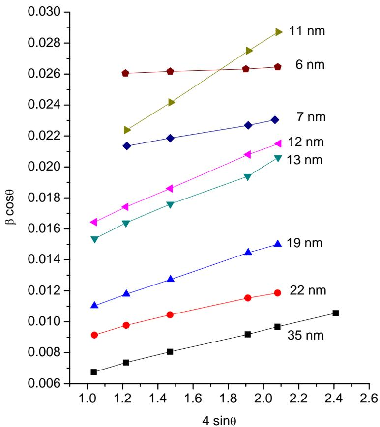
Figure 3: W-H Plot of CrF nanoparticles. Lines are drawn to guide the eyes.
