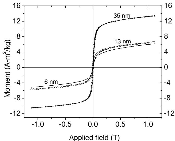
**Figure 6:** Typical M-H curve of 6 nm, 13 nm and 35 nm CrF in an applied field of up to 1.25 T
