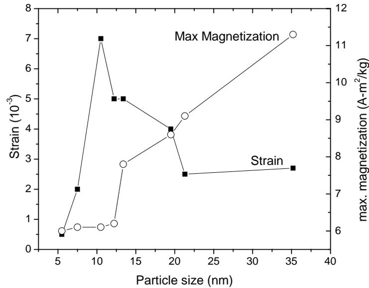
**Figure 4:** Variation of strain and maximum magnetization of CrF nanoparticles with particle size
