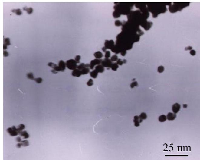
**Figure 5:** Typical TEM micrograph of 11 nm particle size CrF sample
