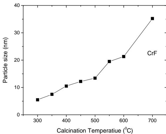
Figure 2: Variation of particle size of CrF with the calcination temperature
