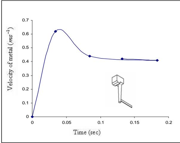
Figure 5: Velocity measurements, flowability filling condition, piece thicknesses 0.75mm, mould Temperature 450°C, pouring Temperature 750°C, and metal head 170mm
