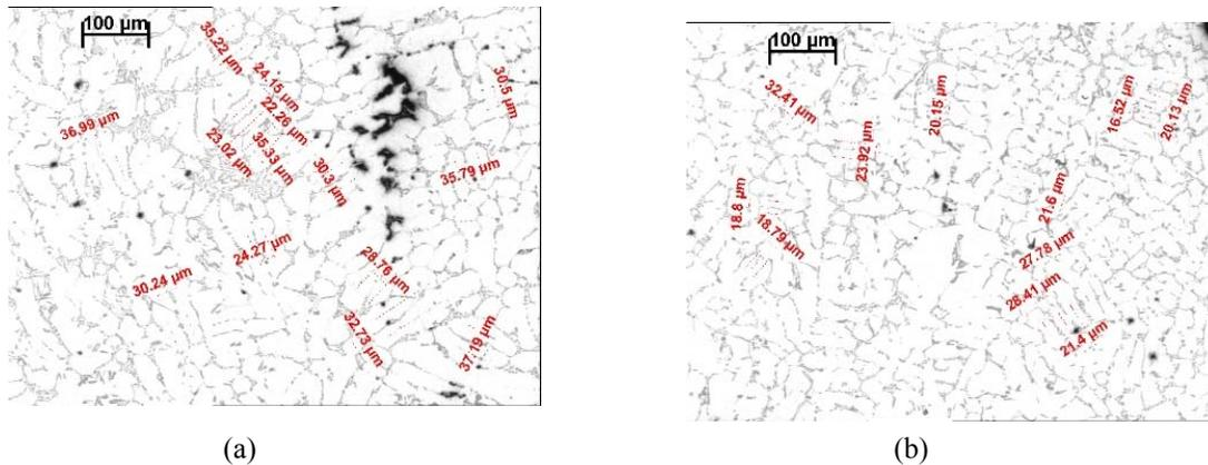
Figure 14 Typical mid-thickness strip microstructures observed at the flow tips of (a) castings filled without vibration and (b) castings filled with 0.8g acceleration (pouring temperature, thickness 0.75mm, 750°C; mould temperature 420°C; metal head 170mm).
