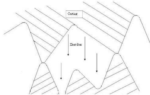
Figure 10: Metal-mould interfaces at the second stage (air gap forming).
