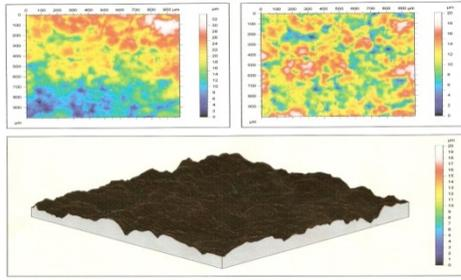
Figure 11 3D-surface roughness profile measured for ceramic mould
