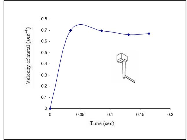
Figure 6 : Velocity measurements, fillability filling condition, piece thicknesses 0.75mm, mould Temperature 660-700°C, pouring Temperature 750°C, metal head 170mm
