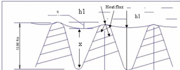
Figure 9: Metal-mould interfaces at the first stage and at the heat flux.
