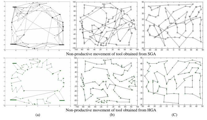
Figure 5. Non Productive Movement of Tool during Machining, Problem Size= (a) (275 Nodes) (b) (150 Nodes) (c) (85 Nodes)
