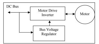
Figure 3. Flywheel Electrical Interface
