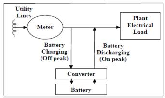
Figure 5. Schematic of a customer-owned LABESS
