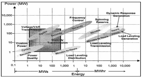
Figure 2. Energy-power characteristics of SMES applications taken from Buckles (2000)
