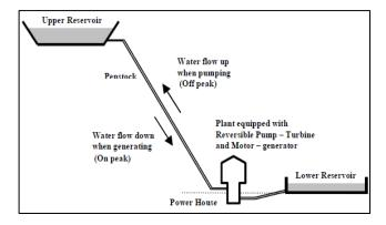
Figure 4. Schematic Diagram of PHESS
