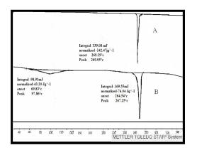
**Figure 2:** DSC thermogram of TP (A) and 20 min cured pellets (B)
