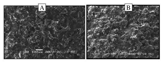
Figure 1: Surface morphology of 5 min (A) and 20 min cured pellets
