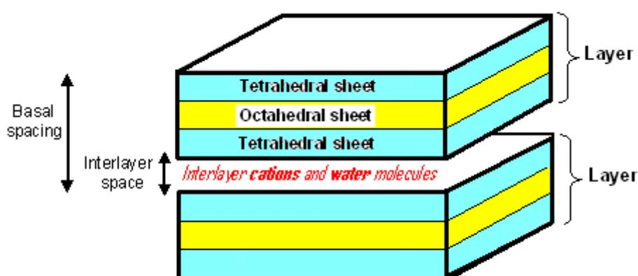
**Fig. 1.** Schematic illustration of montmorillonite clay mineral structure (2:1 type).
