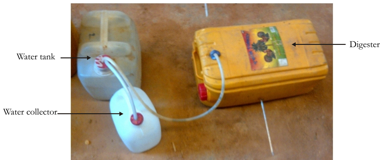
Plate 1. The digester set up
