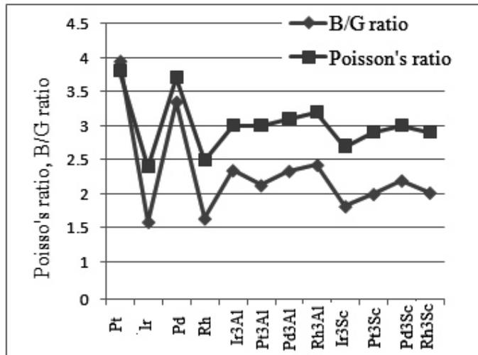
**Figure 2:** Comparison of  $B/G$  and the Poisson's Ratios between Platinum, Iridium, Rhodium and Palladium as well as their alloy with Aluminum or Scandium in the  $L1_2$  Structure. The Poisson's Ratio are Magnified by a Factor of 10
