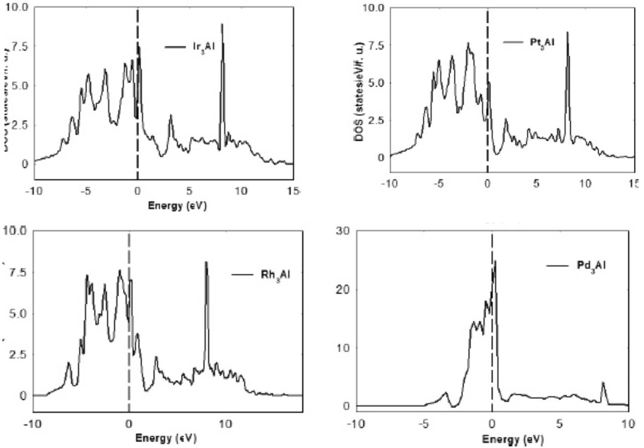
Figure 3: The Total Electronic Density of States for Phases of Iridium with Aluminum ( $\text{Ir}_3\text{Al}$ ), Platinum with Aluminum ( $\text{Pt}_3\text{Al}$ ), Rhodium with Aluminum ( $\text{Rh}_3\text{Al}$ ) and Palladium with Aluminum ( $\text{Pd}_3\text{Al}$ ). Energies Relative to Fermi Level are Indicated by the Dotted Vertical Lines.
