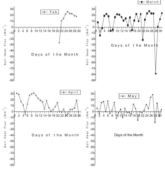
Figure 4(a): Daily Averages of the Soil Heat Fluxes for February to May, 2006 as Measured at the NIMEX Site, Ibadan.
