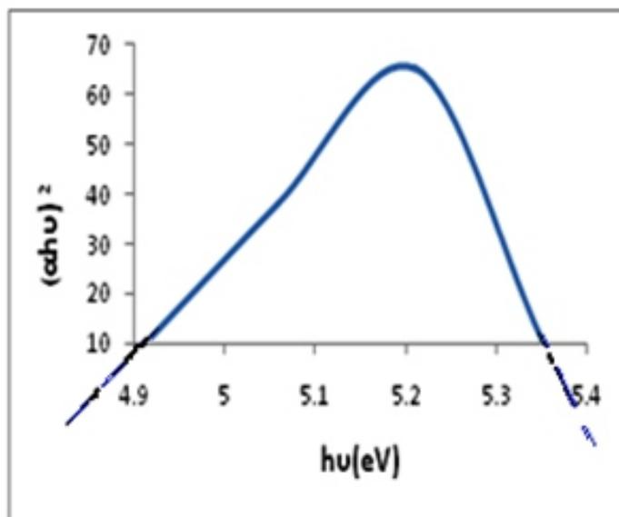
Fig. 9: Dependence of  $(\alpha h\nu)^2$  on the Photon Energy  $h\nu$  for Zn(II) Complex
