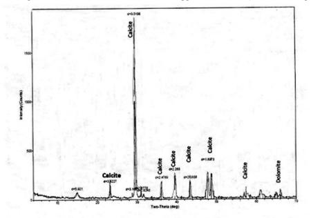
Fig. 3c: X-ray diffraction results of Obajana marble samples
