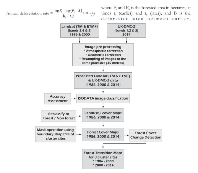
Figure 2: Workflow of Methodology Used for Image Processing
