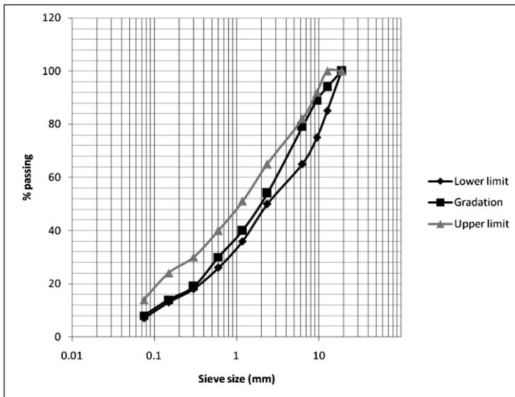
Figure 1: Aggregate Gradation Curve
