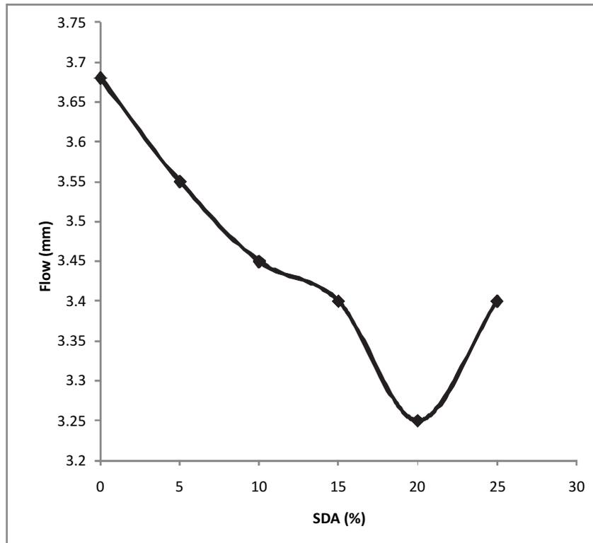
Figure 4: Variation of Flow with Increasing Sawdust Ash (SDA) in the Asphaltic Concrete
