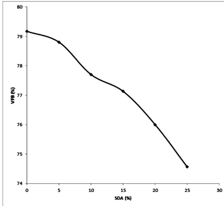
Figure 5: Variation of Voids Filled with Bitumen (VFB) with Increasing Sawdust Ash (SDA) in the Asphaltic Concrete
