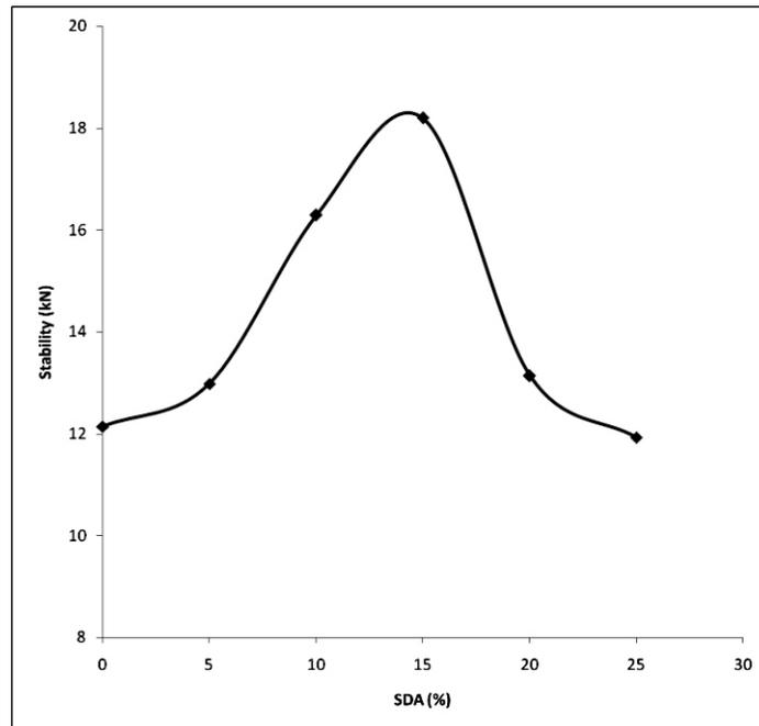
Figure 2: Variation of Stability with Increasing Sawdust Ash in the Asphaltic Concrete
