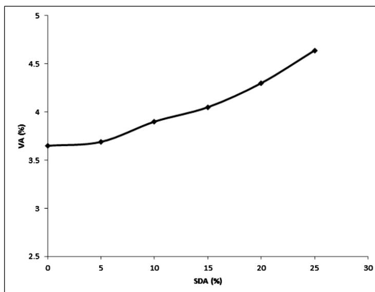
Figure 6: Variation of Air Voids (VA) with Increasing Sawdust Ash (SDA) in the Asphaltic Concrete
