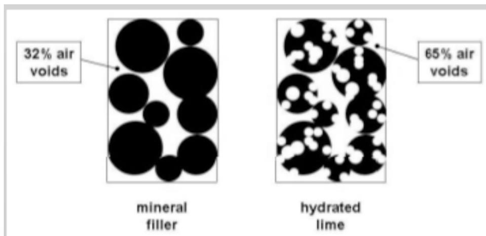
Figure 3: Porosity of Granite and Hydrated Lime Filler Particles
