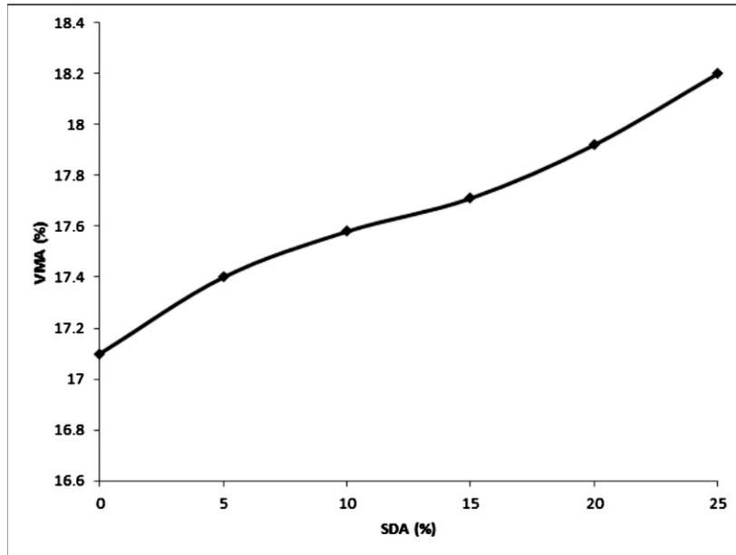
Figure 7: Variation of Voids in Mineral Aggregate (VMA) with Increasing Sawdust Ash (SDA) in the Asphaltic Concrete
