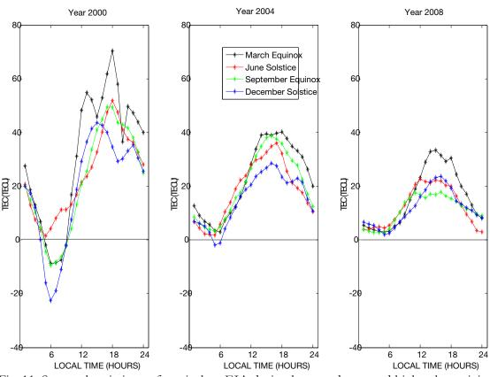
Fig. 11: Seasonal variations of equivalent EIA during low, moderate and high solar activity.
