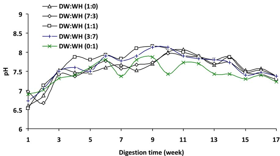
Figure 2. Profile of Substrate pH during Digestion
