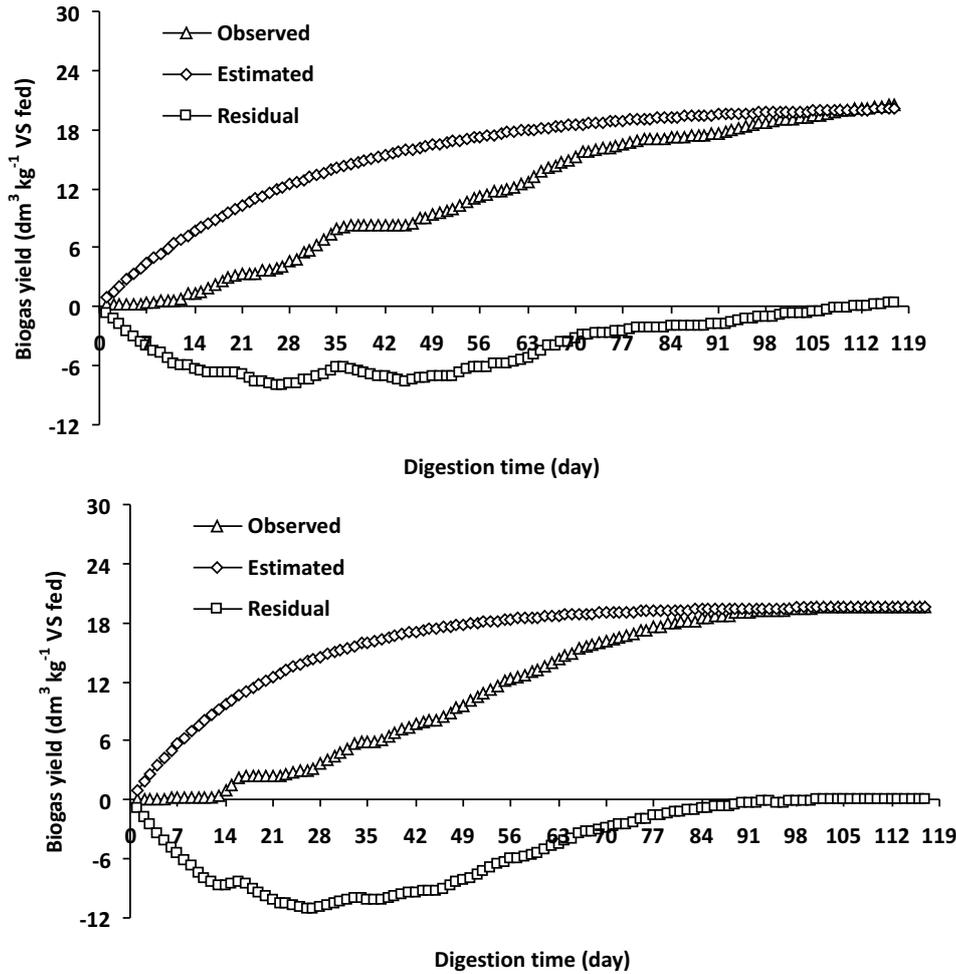
Figure 5. Profile of Observed and Estimated Cumulative Biogas Yield: a) DW:WH (1:0), b) DW:WH (7:3), c) DW:WH (1:1), d) DW:WH (3:7) and e) DW:WH (0:1) Residual = Observed - Estimated. DW, duck weed; WH, water hyacinth; VS, volatile solids
