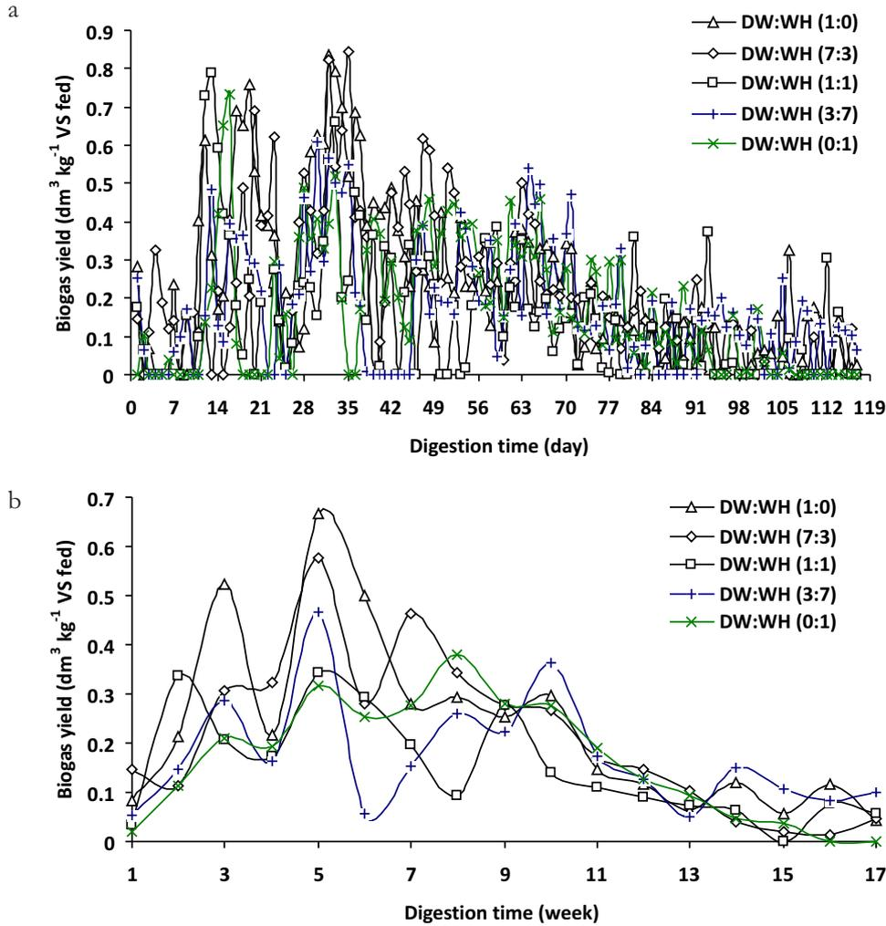
Figure 4. Profile of Biogas Yield (a) Daily and (b) Weekly
