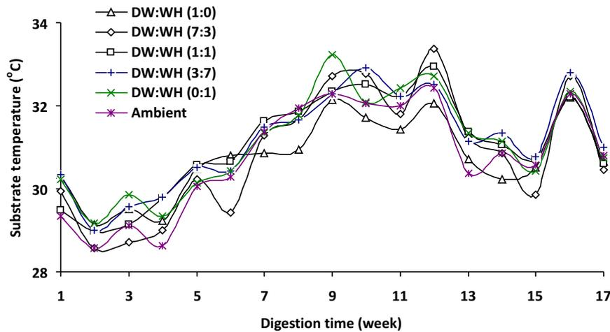
Figure 1. Profile of Substrate Temperature during Digestion
