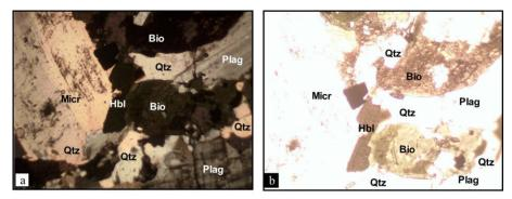
Figure 12: Thin section photomicrographs of porphyitic granite (Magnification: 100x). (a) Under crosspolarised light (b) Under plane-polarised light.
