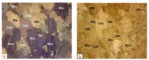
Figure 9: Thin section photomicrographs of cal-silicate gneiss (Magnification: 100x). (a) Under crosspolarised light (b) Under plane-polarised light.
