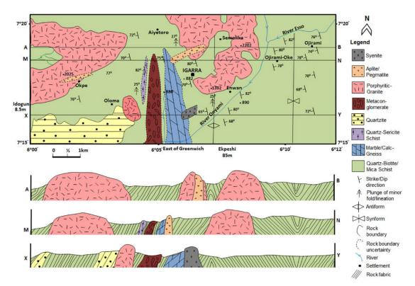
Figure 2: Geological map of Igarra and surrounding areas with cross sections indication lines of section AB, MN and XY.
