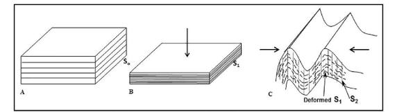
**Figure 20:** Simplified sketch of the structural model of the metasediments in Igarra and surrounding areas, Southwestern Nigeria. (A) Original sedimentary layer (S<sub>0</sub>). (B) The deformation of S<sub>0</sub> to S<sub>1</sub> as a result of gravitational stress, S<sub>1</sub> is parallel to S<sub>0</sub>. (C) The formation of S<sub>2</sub> is then formed as a result of horizontal compression.
