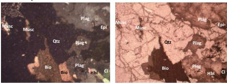
Figure 6: Thin section photomicrographs of metaconglomerate (Magnification: 40x). (a) Under crosspolarised light (b) Under plane-polarised light.
