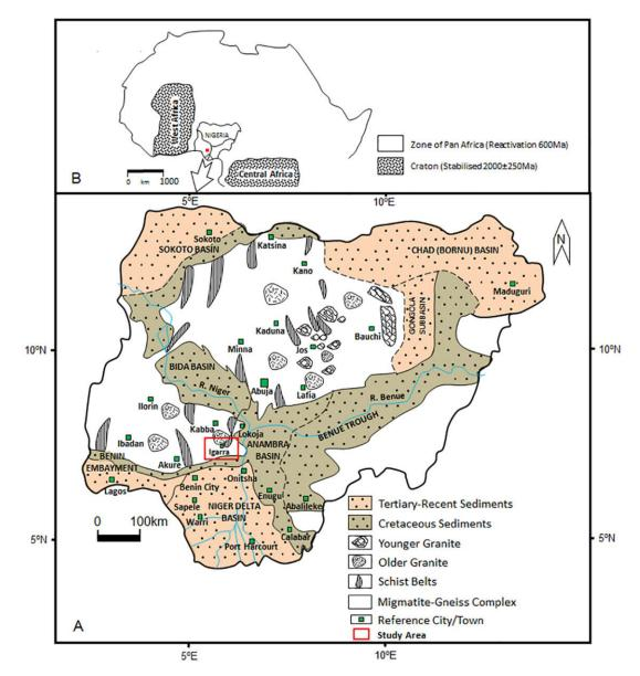
Figure 1 Simplified geologic map of Nigeria showing the study area (A). Inset is the map of Nigeria within the African shield (B)
