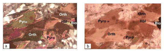
Figure 14: Thin section photomicrographs of metaconglomerate (Magnification: 100x). (a) Under cross-polarised light. (b) Under plane-polarised light.
