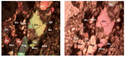
Figure 4: Thin section photomicrographs of quartz-biotite schist (Magnification: 40x). (a) Under crosspolarised light. (b) Under plane-polarised light.
